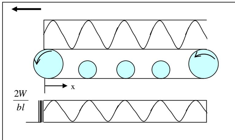
**Figure (4) Case 4: Sinusoidal normal pressure distribution**
