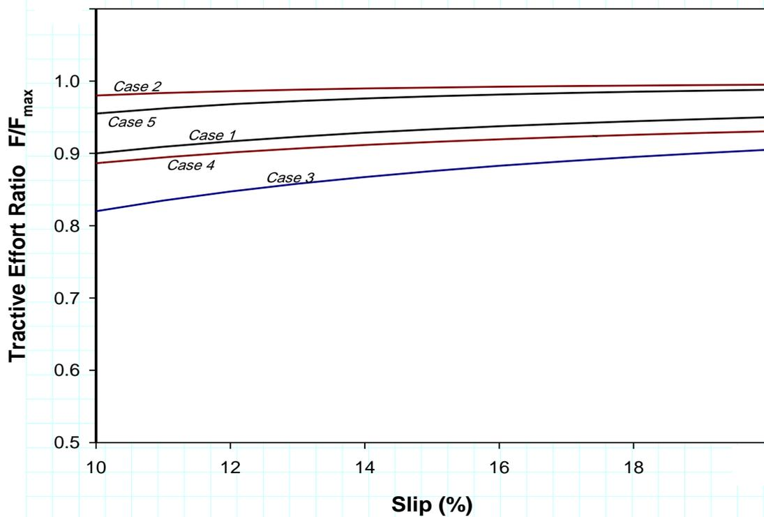
Figure (8) Tractive effort ratio against slip for the normal slip range
