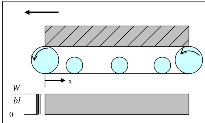
Figure (1) Case1: Uniform normal pressure distribution
