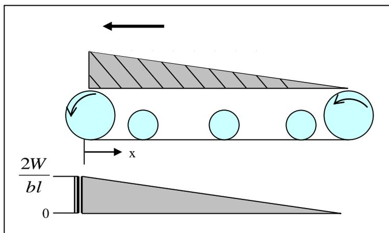
Figure (3) Case 3: Normal pressure decreasing linearly from front of vehicle
