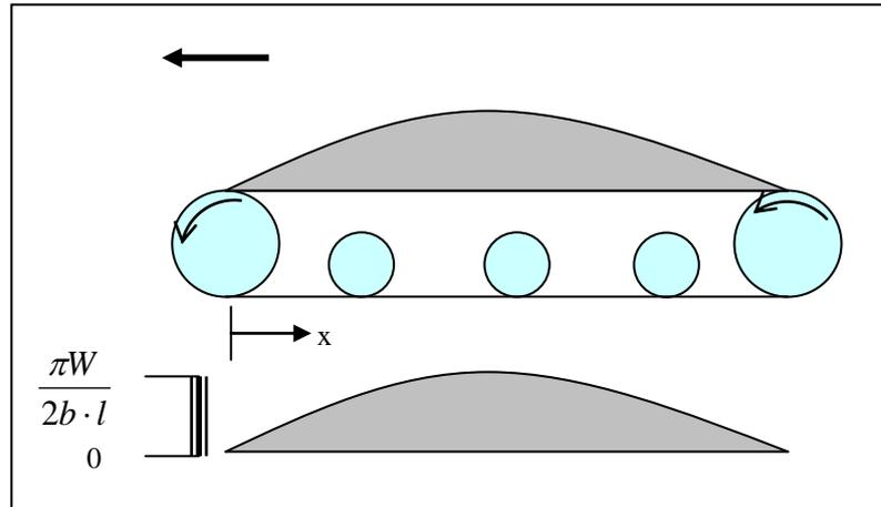
Figure (5) Case 5: Sinusoidal normal pressure distribution with maximum pressure at the center and zero pressure at the front and rear ends
