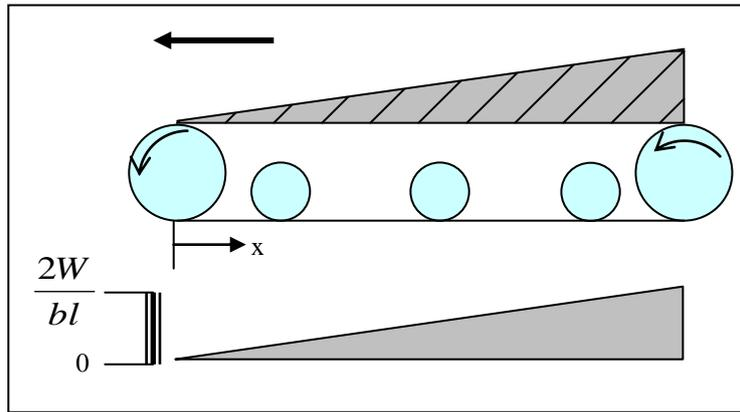
Figure (2) Case 2: Normal pressure increasing linearly from front of vehicle
