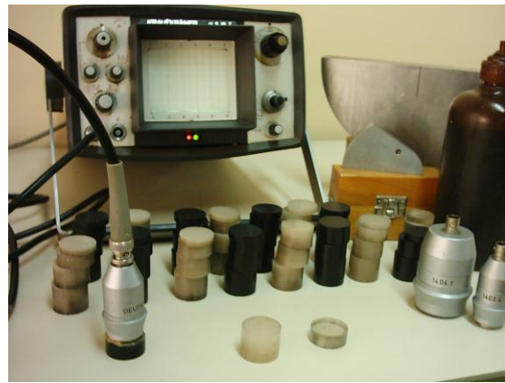
Figure (4) Krautkramer ultrasonic flaw detector USM2 type and test samples
