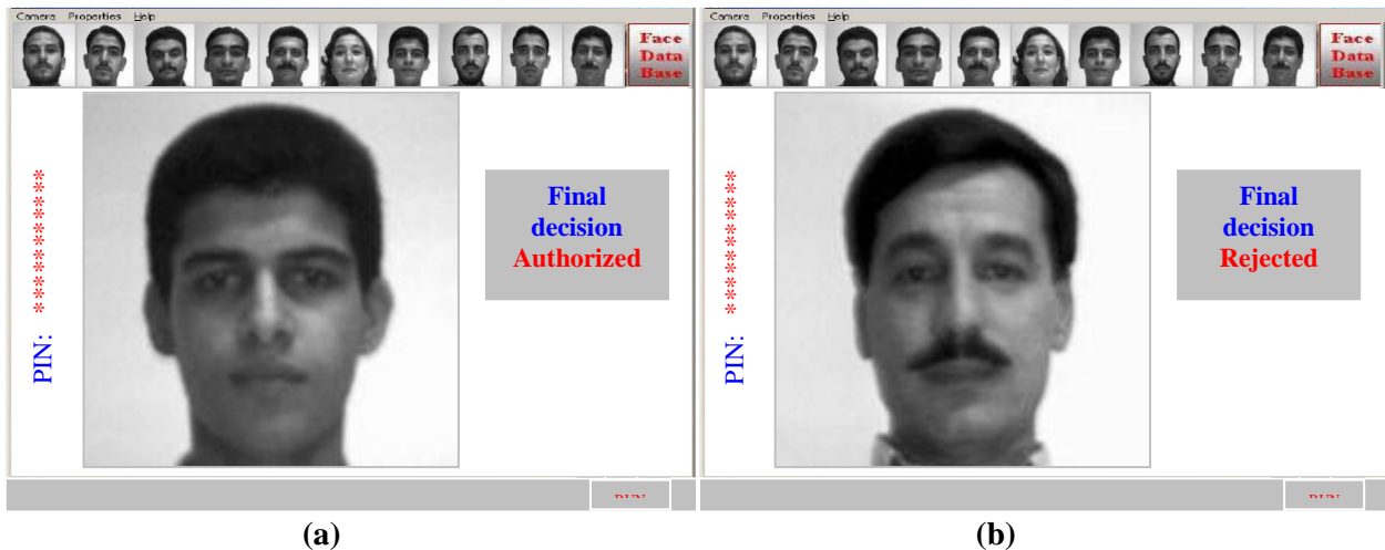
Figure (8) Examples where: (a): An authorized person is recognized. (b): An intruder to the system is rejected. With sample faces of database
