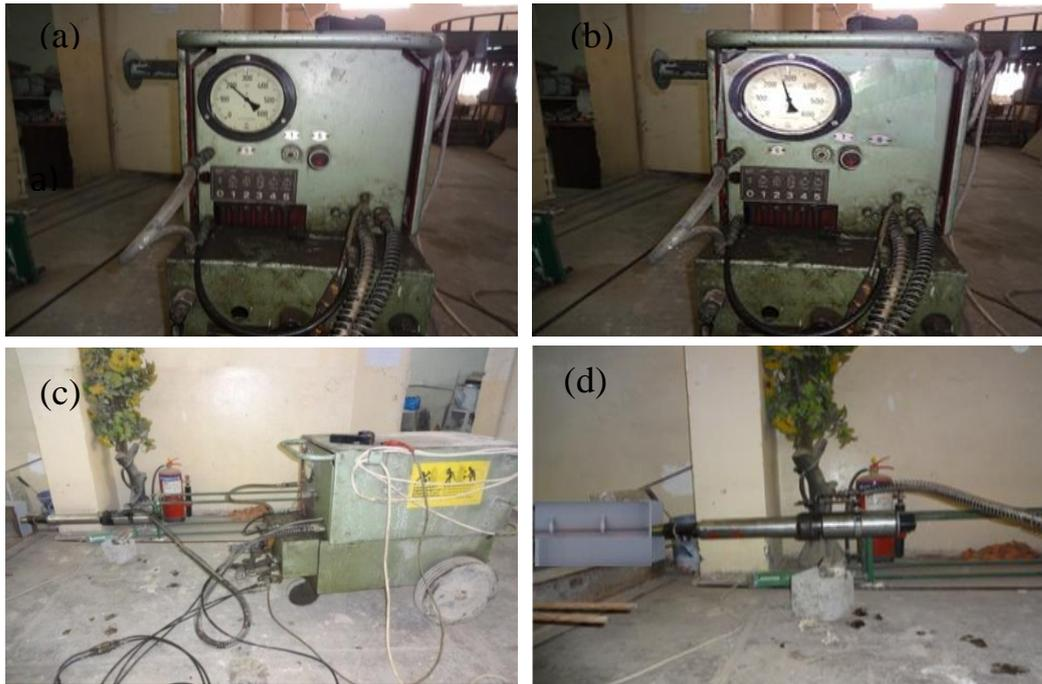
Plate (6) Hydraulic machine and single strand jack prestressing strand. (a) Hydraulic machine and measuring gauge at (200 bar), (b) Hydraulic machine and measuring gauge at (275 bar), (c) the single strand jack and Hydraulic machine with hydraulic pipes attached to the four hydraulic jacks, (d) single jacking prestressing strand.
