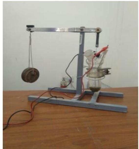
**Figure 2.** Illustrated the static stress corrosion cracking device that designed and manufactured locally according to the American Standard (ASTM G103 - 97) [15].
