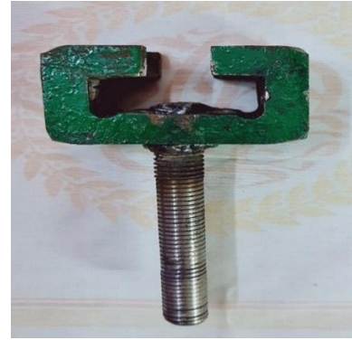
Figure 3. The manufactured fixture according to ASTM A370-14
