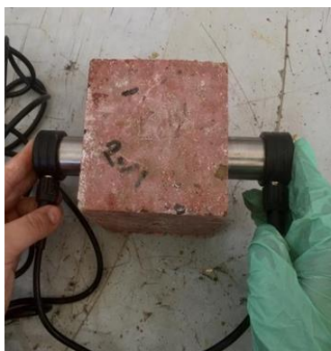
Figure 5. Ultrasonic Pulse Velocity direct test
