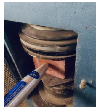
Figure 3. Rebound number test.
