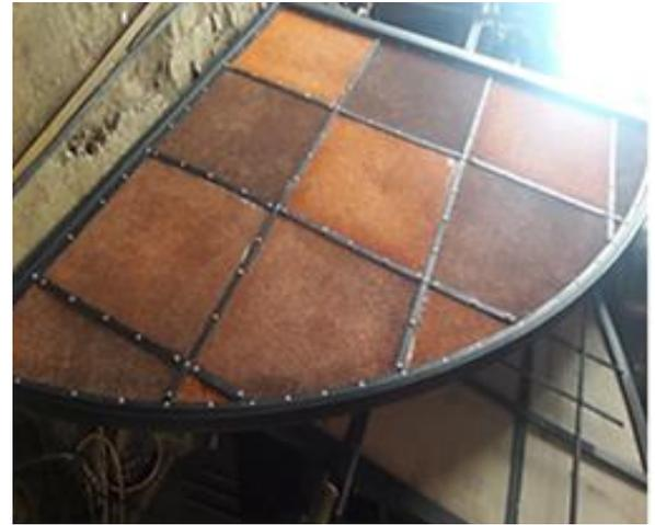
**Figure 8.** Final design of copper foam absorption plate
