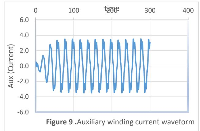
**Figure 9.** Auxiliary winding current waveform
