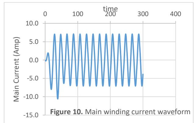
**Figure 10.** Main winding current waveform
