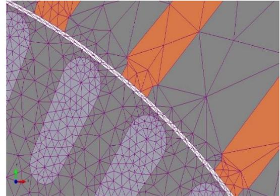
Figure 2. Enlarged view of air gap meshing
