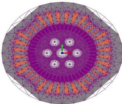
Figure 1. Test motor model meshing by magnet
