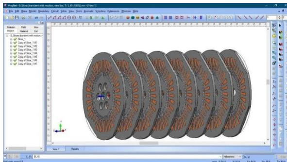
Figure 4. Divided of model in to 8 slices using Magnet software
