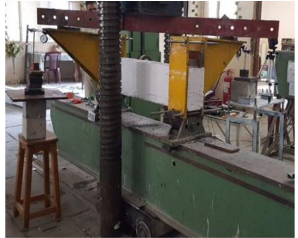
Figure 8. Installation Tested Beam
