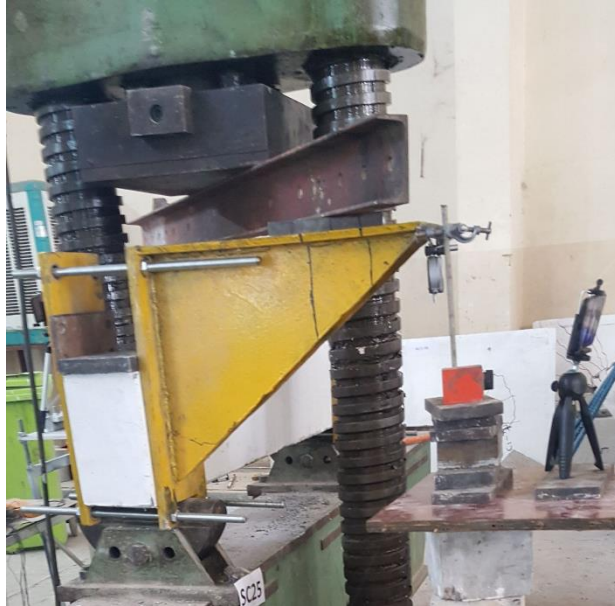
Figure 7. Dial Gauge Located
