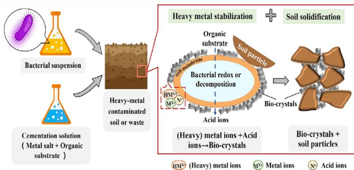
Figure2. Process of soil bioremediation by MICP
