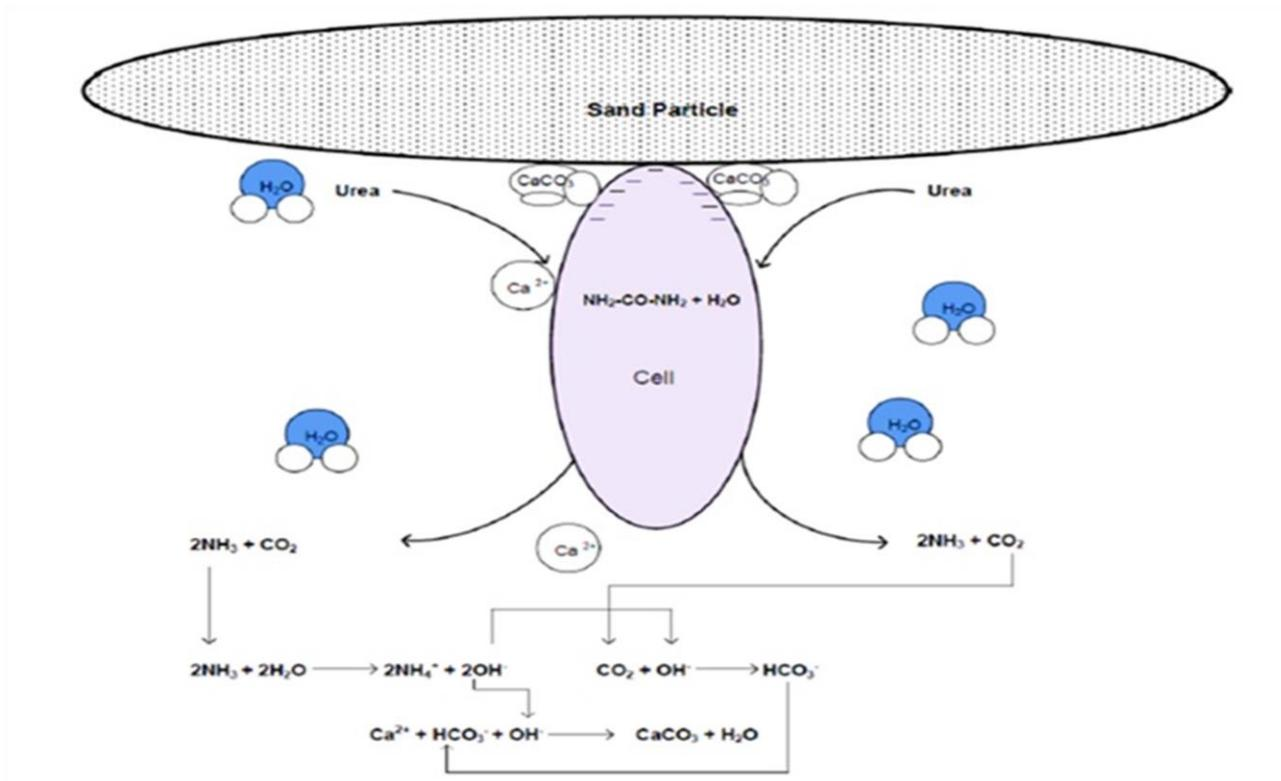
**Figure 1.** Depicts the overall chemical reaction process that takes place in the soil matrix
