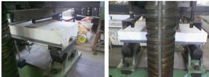
Figure (3) Loading set up and measuring devices
