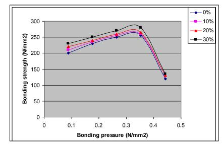
Figure (3) Bonding pressure vs tensile strength of diffusion bonded joints Cu-Ni for different plastic deformation
