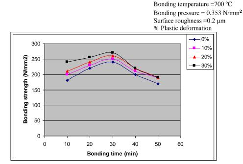
Figure (2) Bonding time vs tensile strength of diffusion bonded joints Cu-Ni for different plastic deformation
