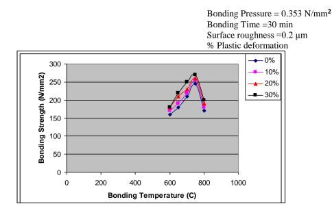
Figure (1) Bonding temperature vs tensile strength of diffusion bonded joints Cu-Ni for different plastic deformation
