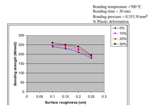
Figure (4) Surface roughness vs tensile strength of diffusion bonded joints Cu-Ni for different plastic deformation
