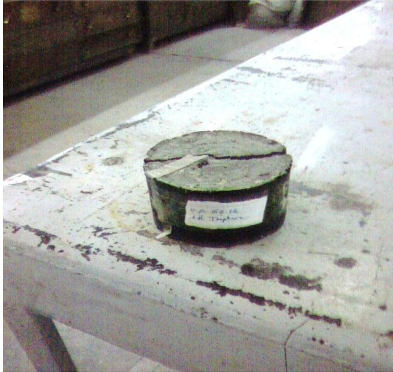
Plate (13): Images of Failed Specimen.
