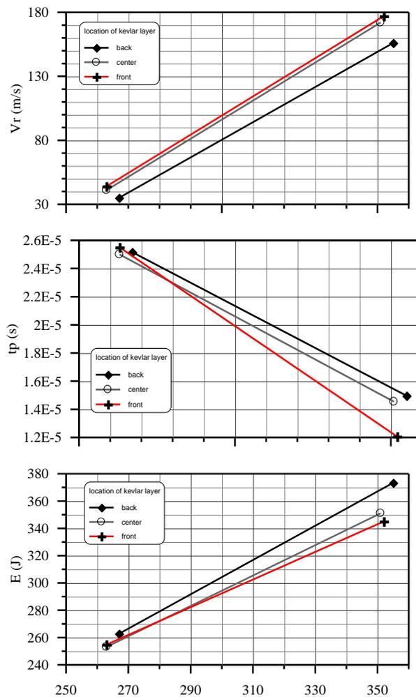
**Figure (9) The Impact experimental results of verses incident velocity for hybrid composites of 10 layers plain E-Glass with different location of Kevlar layer (fiber reinforced polyester composite)**
