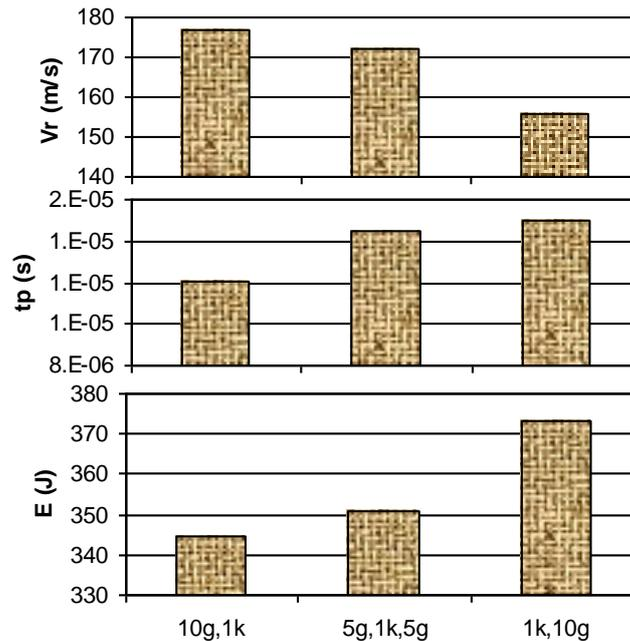
Figure (10) The Impact experimental results verses location of Kevlar layer for hybrid composites of 10layers plain E-Glass with different location of Kevlar layer (fiber reinforced polyester composite) for  $V_i \sim 350$ m/s
