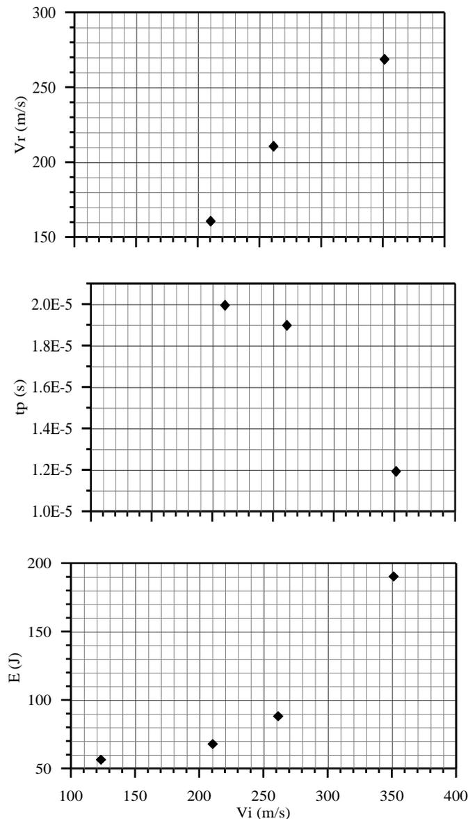
Figure (4) The impact experimental results of the 10-layers p1gp ( $h=3.9\text{mm}$ ), impacted by  $60^\circ$ , 7.5 g steel projectile for various incident velocities
