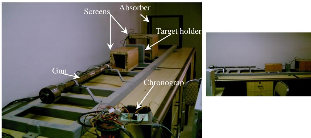
**Figure (3) Photographic view of the presented impact rig**
