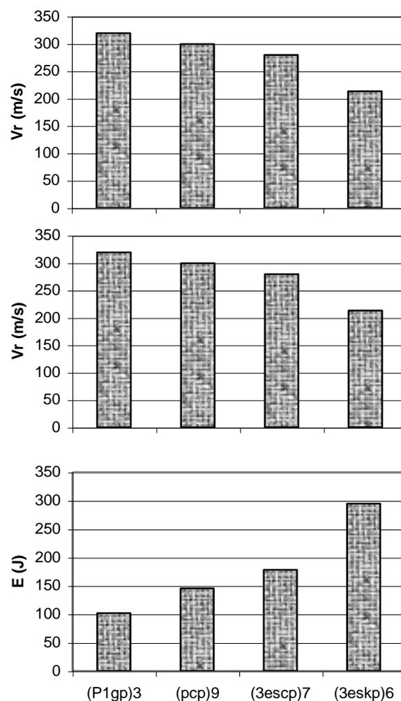
**Figure (8) The Impact experimental results of the ( $h \sim 1.4\text{mm}$ ), impacted by 60o, 7.5 g and ( $V_i \sim 350$ ) projectile for various composite materials)**
