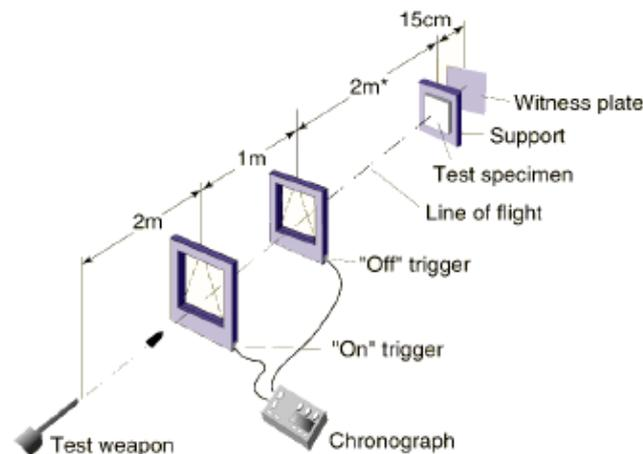
**Figure (1) Ballistic testing {National Institute of Justice (NIJ) standards}**<sup>[13]</sup>
