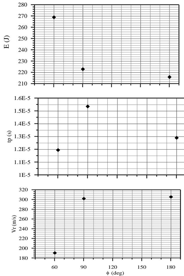
Figure (5) The Impact experimental results of the 10-layers p1gp (h=3.9mm), impacted by 7.5 g ( $V_i \sim 353$ m/s) steel projectile with various nose angles
