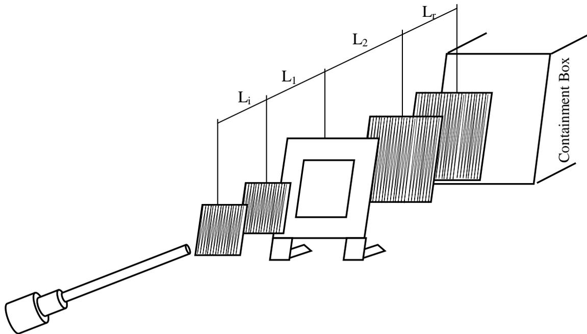
**Figure (2) Schematic representation of the ballistic rig**
