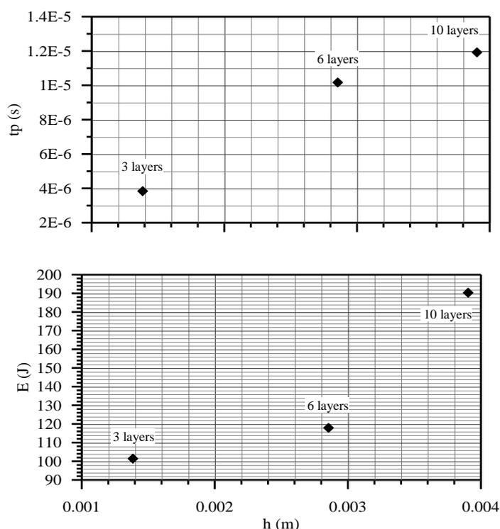
**Figure (6) The Impact experimental results of p1gp, impacted by 7.5 g (Vi=353m/s) steel projectile with various thickness (No of layers)**
