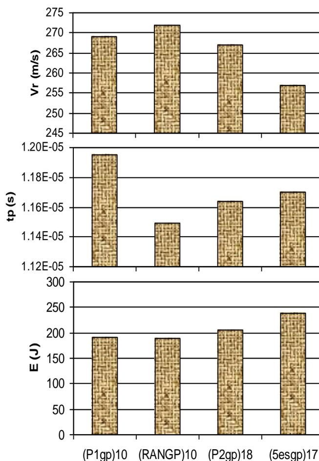
**Figure (7) The Impact experimental results of the ( $h \sim 4\text{mm}$ ), impacted by 600, 7.5 g and ( $V_i \sim 350$ ) projectile for various weave style of glass reinforced polyester**
