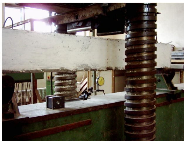
Plate (1) Set-Up of beam specimen test
