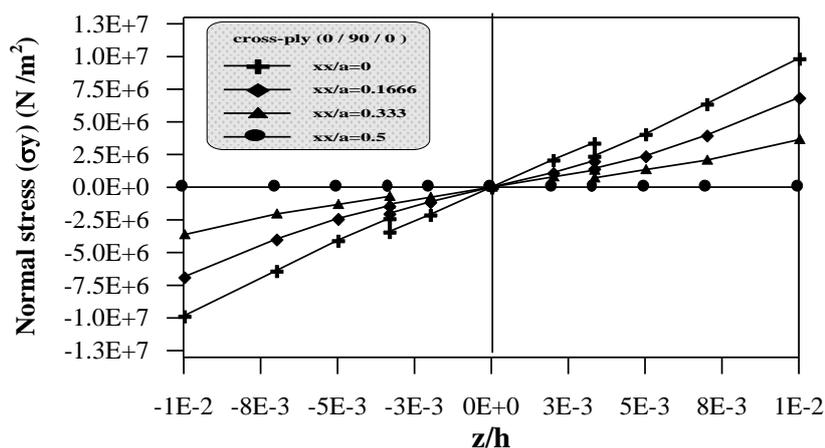
Figure (10) Stress distribution  $\sigma_y$  through the thickness
