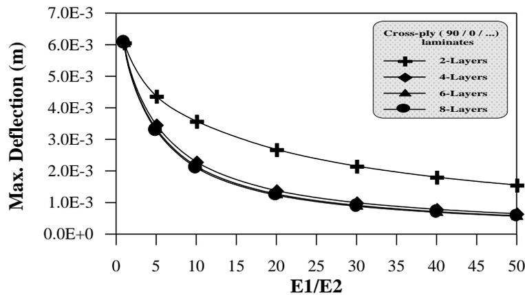
Figure (3) Effect of orthotropic ratio on a maximum deflection of a square antisymmetric cross-ply laminated plate (V=10 m/sec)
