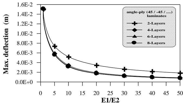
Figure (4) Effect of orthotropic ratio on a maximum deflection of a square antisymmetric angle-ply laminated plate (V=20 m/sec)
