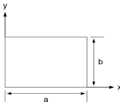
Figure (1) Geometry and the co-ordinate system of a rectangular plate
