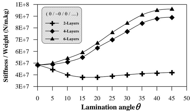
**Figure (8) Effect of lamination angle on the stiffness-to-weight ratio of antisymmetric angle-ply laminates**
