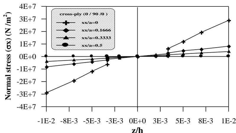
**Figure (9) Stress distribution  $\sigma_x$  through the thickness**
