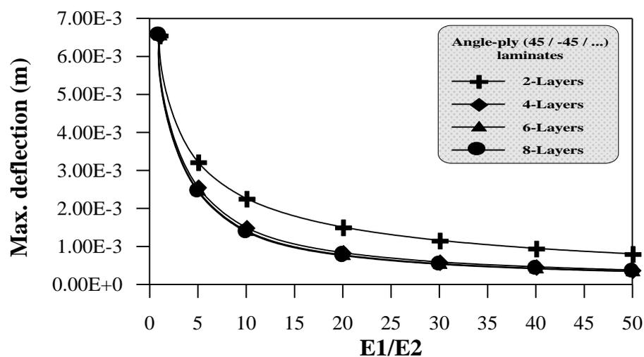
Figure (2) Effect of orthotropic ratio on a maximum deflection of a square antisymmetric angle-ply laminated plate ( $V=10 \text{ m/sec}$ )
