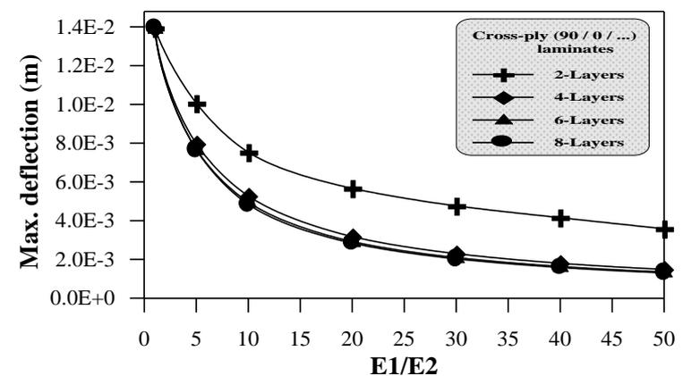
Figure (5) Effect of orthotropic ratio on a maximum deflection of a square antisymmetric cross-ply laminated plate (V=20 m/sec)
