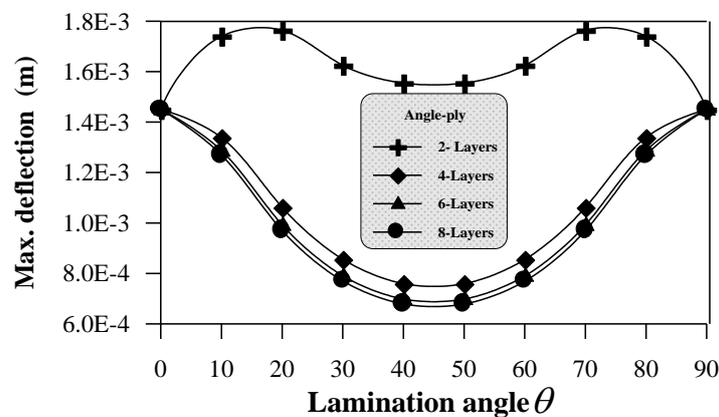
Figure (6) Effect of lamination angle on a maximum deflection of a square antisymmetric angle-ply laminated plate ( $V=15$  m/sec)
