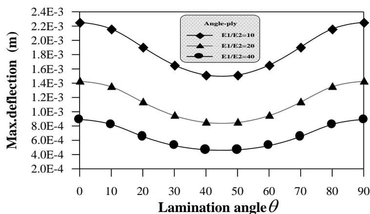
**Figure (7) Effect of lamination angle and orthotropic ratio on a maximum deflection of a square antisymmetric angle-ply laminated plate (V=10 m/sec)**
