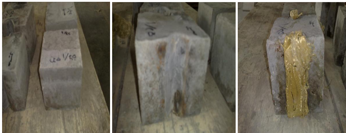
Fig.(4) A. solid sample B. sample have notch C. repair sample with Kevlar .
