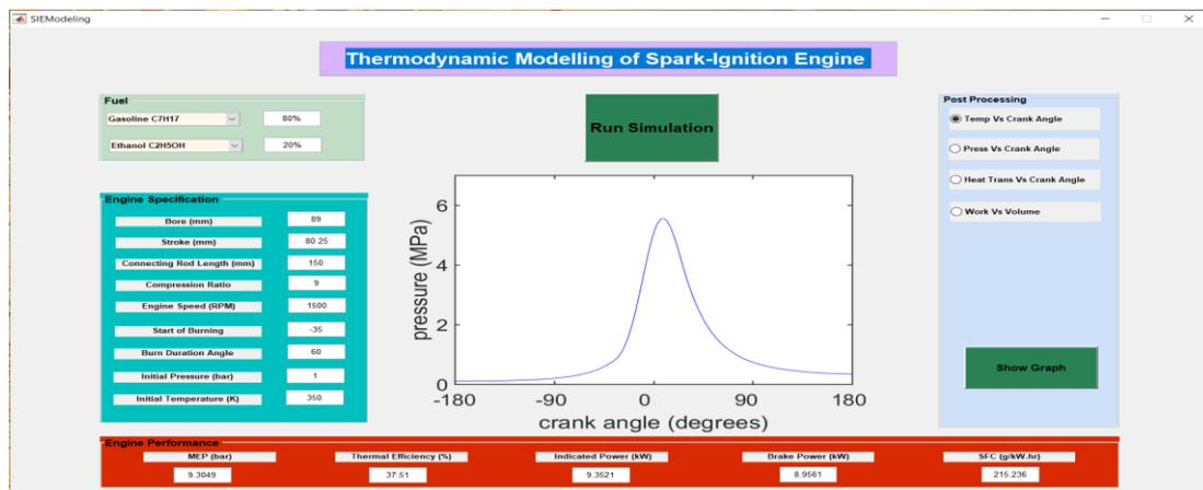
Figure 2. MATLAB interface of the SI engine simulation program.
