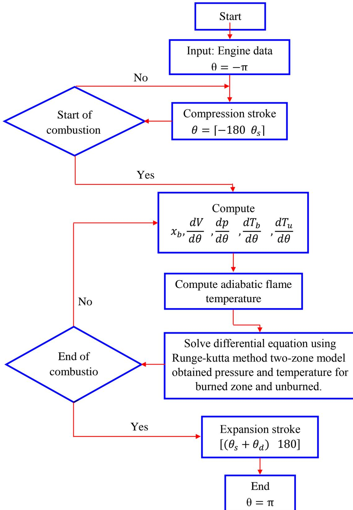
Figure 3. Solution procedure of the combustion of two zone (SI) engine model
