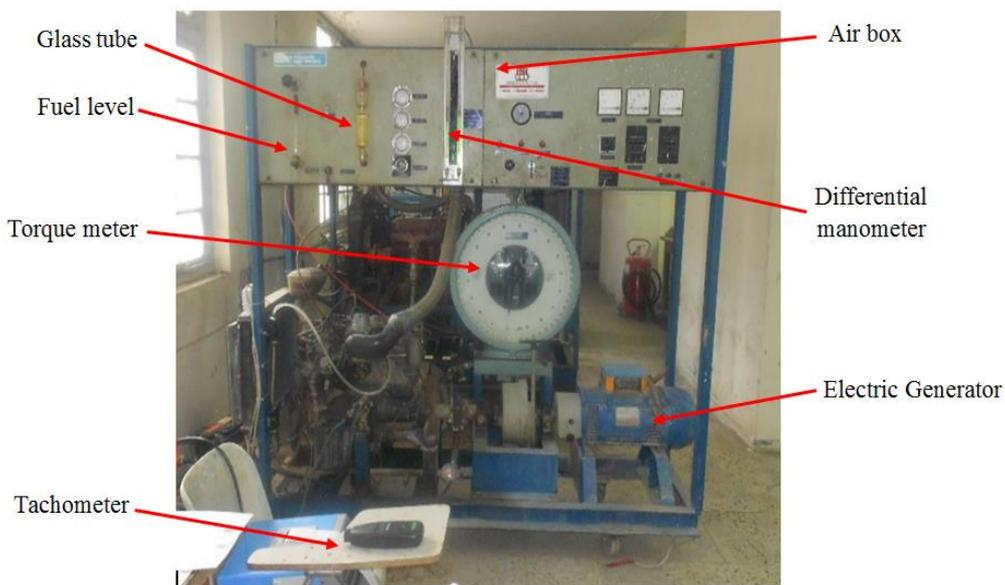
Figure 4 .The experimental setup of (S.I. engine)
