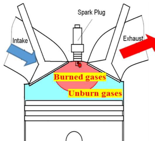
Figure1. Two-zone thermodynamic model of combustion
