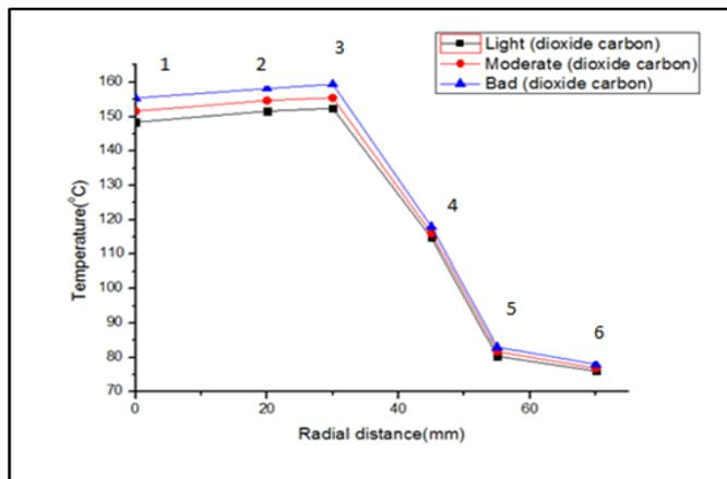
Figure 9. Temperature of each motor part at different contamination levels.
