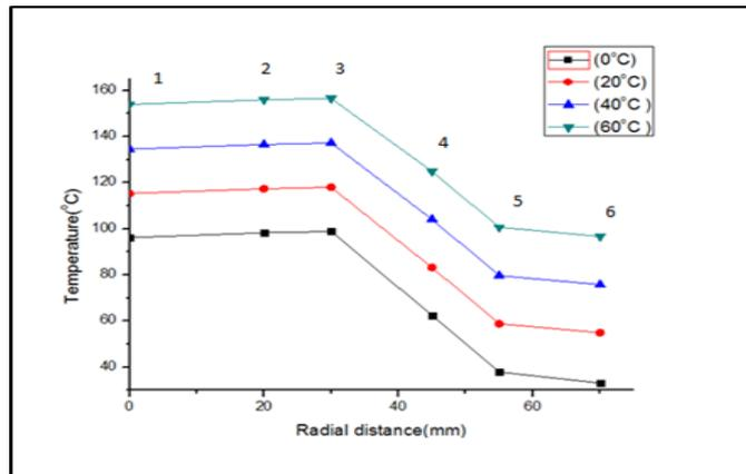
Figure 6. Temperature of each motor part at different ambient temperature
