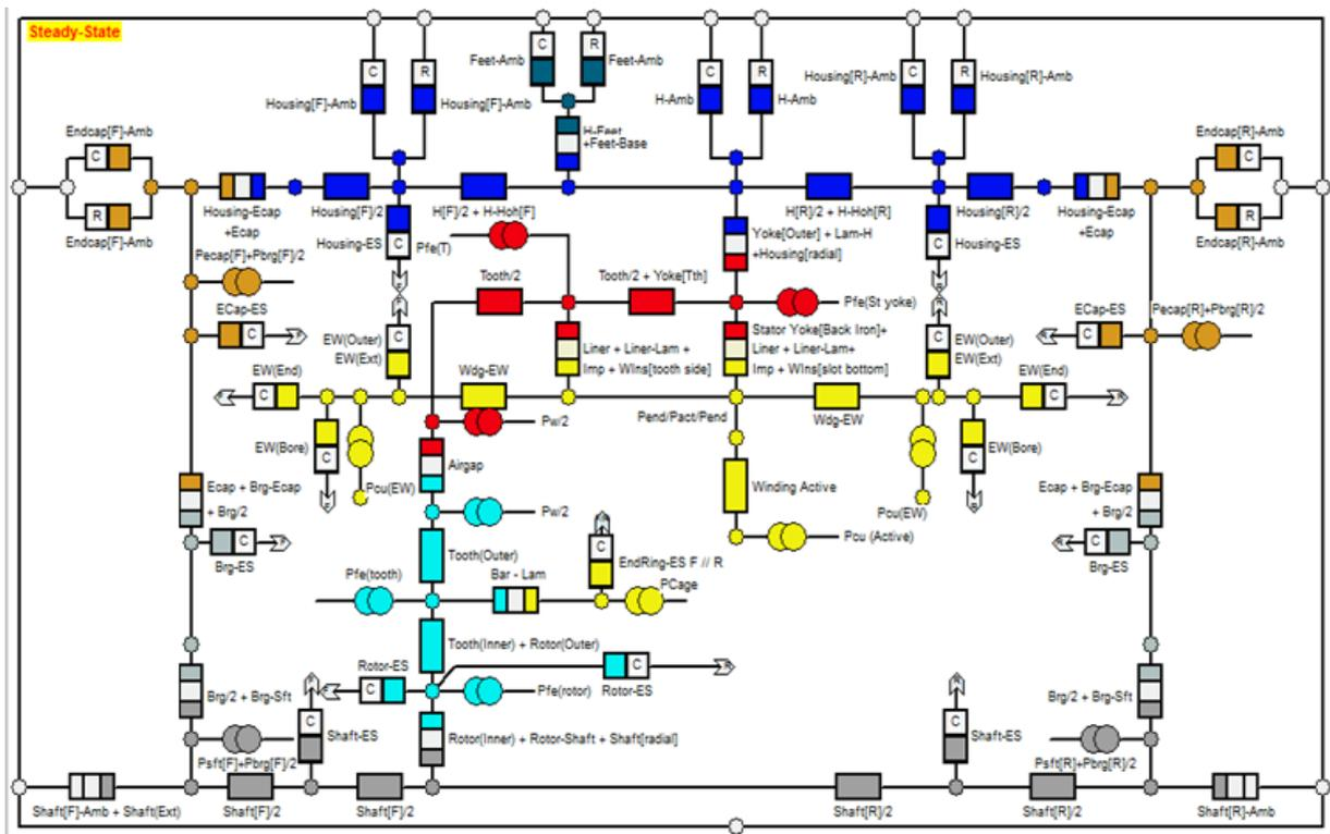
Figure 3. Equivalent thermal network of the test motor by Motor-CAD
