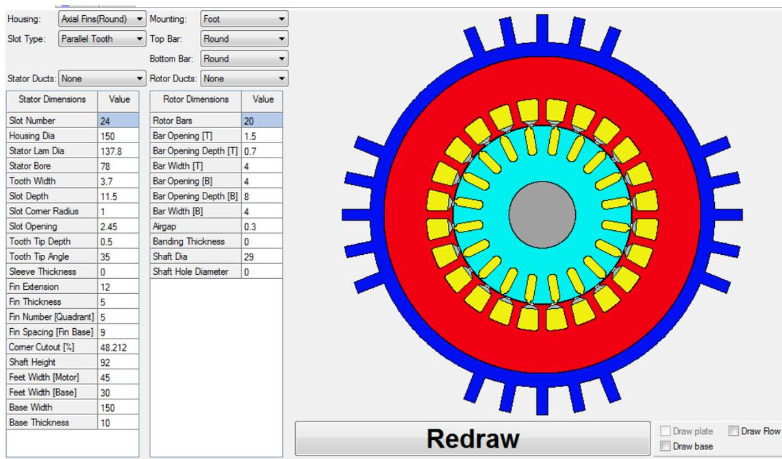
Figure1. Radial dimension of the test motor by Motor-CAD.
