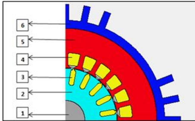
Figure 5. Motor six regions for temperature estimation
