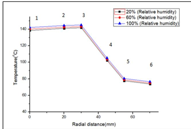
Figure 8. Temperature of each motor part at different relative humidity
