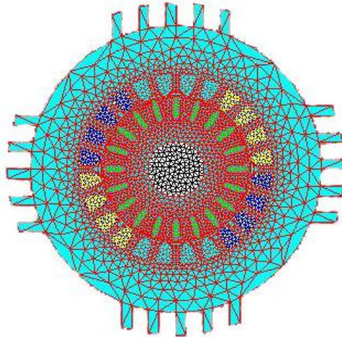
Figure 4. FEM model for the test motor by Flux2D
