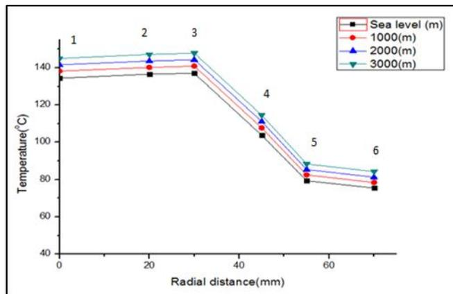
Figure 7. Temperature of each motor part at different altitude
