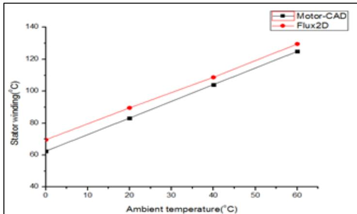
Figure 10. Comparison of stator winding temperature estimated by Motor-CAD and Flux2D.
