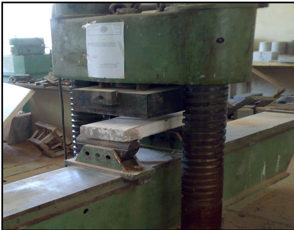
Fig (11) The Machine Applied Load On The Slab (Structural Laboratory In College Of Engineering In Al- Mustansirya University)
