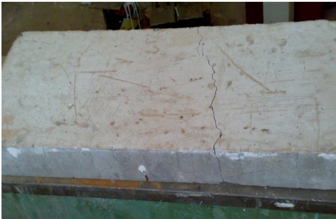
Fig (12) Deflected Slab
