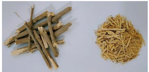
**Figure 1.** Sesbania stems before and after grinding
