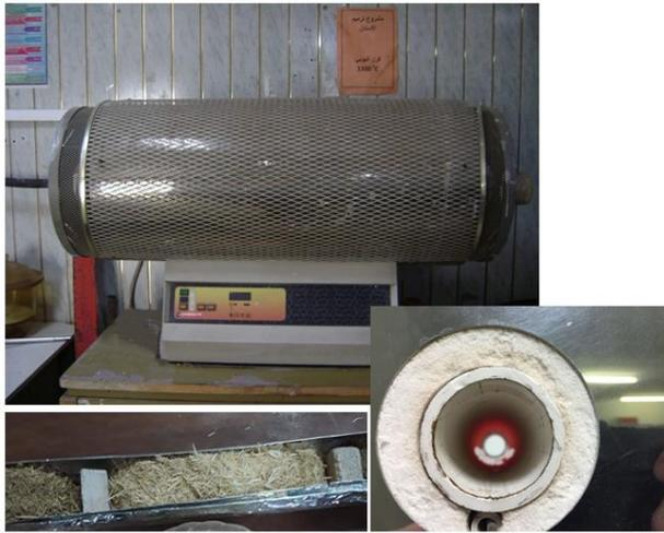
**Figure2.** CARBOLITE Laboratory Horizontal Tube Furnace and the alumina boat (Pyrolysis process).
