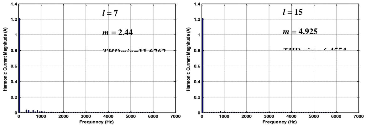
Fig. 10: the Line Current Spectra of Motor Fed by OHESW Cascade Multilevel Inverter at THDmin with Two Values of  $l$
