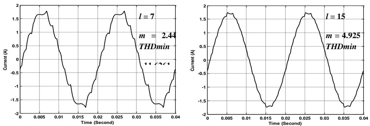
Fig. 9: the Instantaneous Current of Motor Fed by OHESW Cascade Multilevel Inverter at THDmin with Two Values of  $l$
