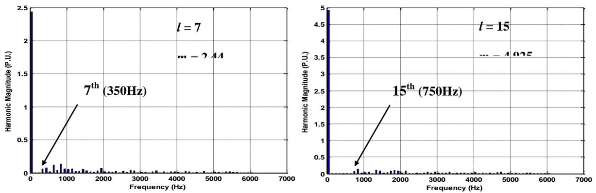
Fig. 8: the Harmonic Content of OHESW for Cascade Multilevel Inverter at THDmin with Two Values of  $l$
