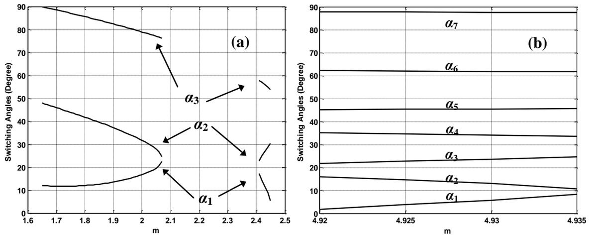
Fig. 4: the Solution of Switching Angles vs.  $m$  for Cascade Multilevel Inverter using OHESW Technique with (a)  $l=7$  and (b)  $l=15$
