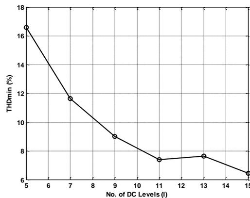
Fig. 6: the Lowest Voltage THD vs. Number of Voltage Levels ( $l$ ) for Cascade Multilevel Inverter using OHESW Technique
