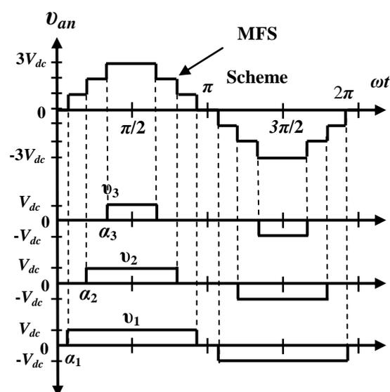
**Fig. 2 : Voltage Output of Cascaded H-bridges Multilevel Inverter**
