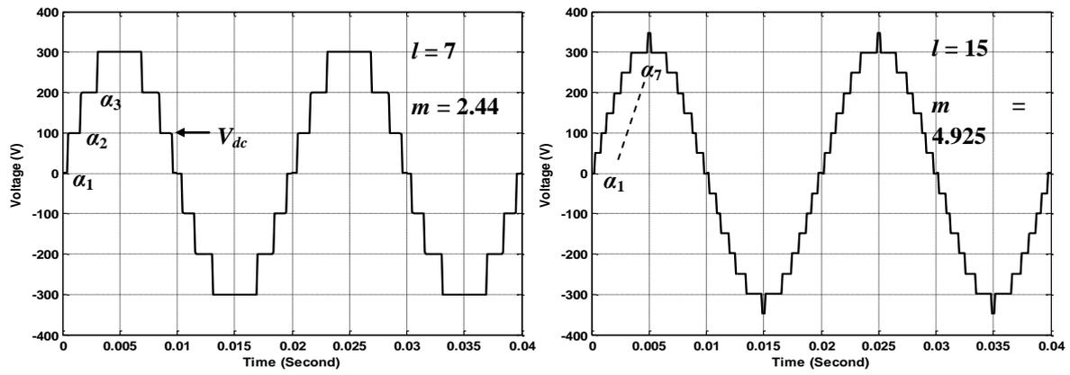
Fig. 7: the Instantaneous Voltage of OHESW Cascade Multilevel Inverter at THDmin with Two Values of Voltage Levels ( $l$ )
