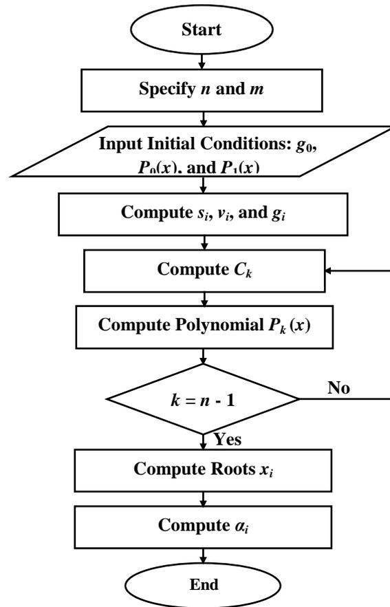
**Fig. 3: Flowchart of a Fast Recursive Algorithm for OHESW Technique**
