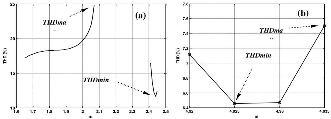
Fig. 5: the Voltage THD vs.  $m$  for Cascade Multilevel Inverter using OHESW Technique with (a)  $l=7$  and (b)  $l=15$
