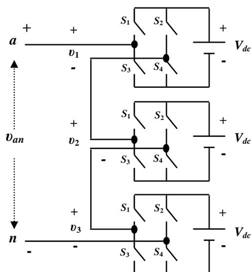
**Fig. 1: Cascaded H-bridges Multilevel Inverter using 3-DC Sources**
