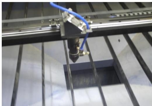
Figure(2): Laser drilling head.
