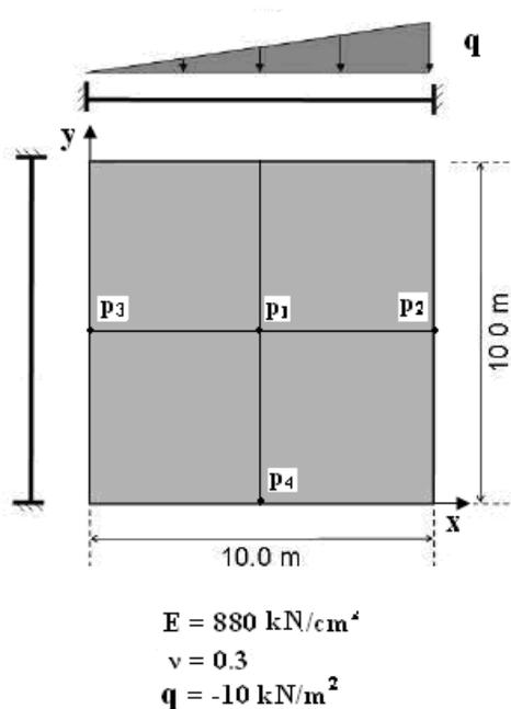
Figure (4): A square plate with clamped edges.
