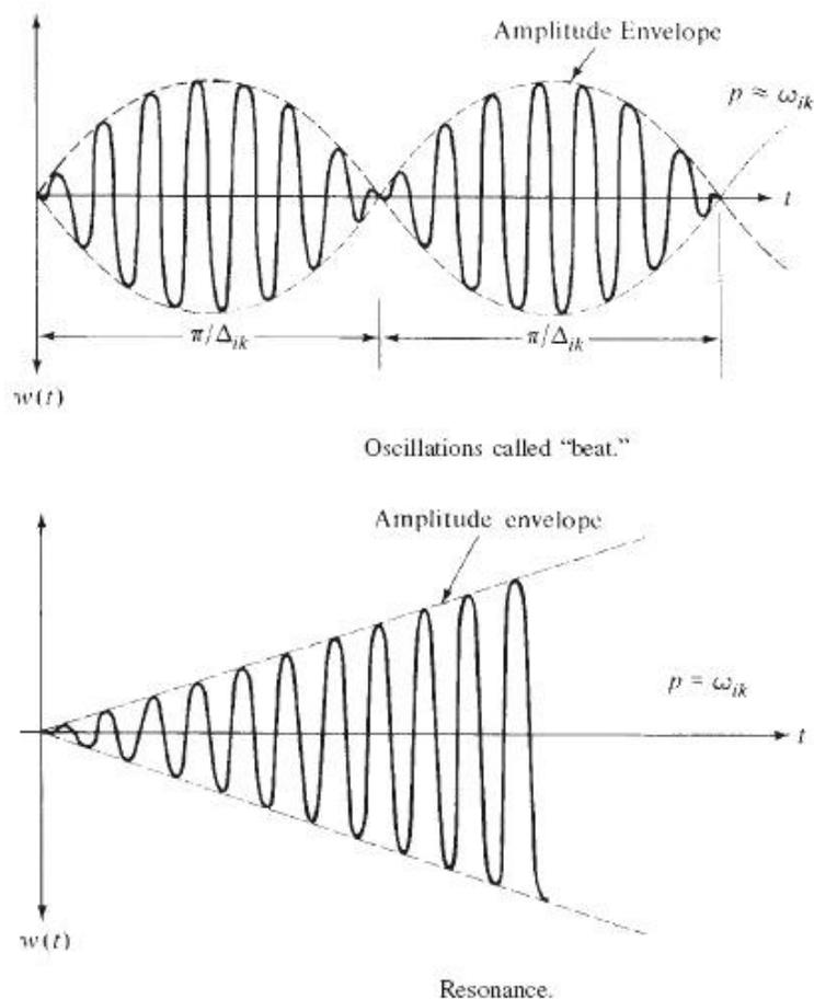
**Figure (2): The general nature of resonance condition phenomenon <sup>(5)</sup>.**
