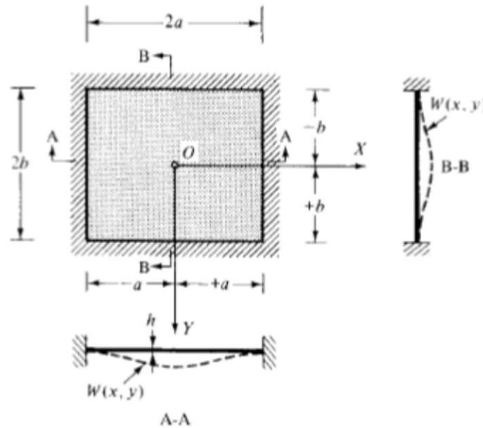
Figure (3): A rectangular plate clamped on all edges.
