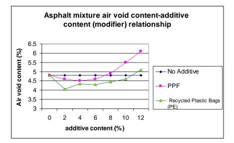
Figure (4) Asphalt Mixture Air Void Content – Additive Content (Modifier) Relationship.
