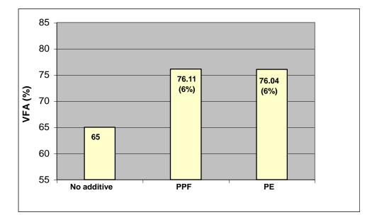
Figure (10) Maximum Asphalt Mixture Void Filled with Asphalt (VFA %) by Type of Modifier.
