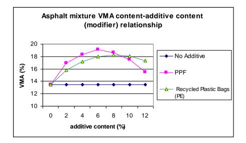
Figure (5) Asphalt Mixture VMA Percentage – Additive Content (Modifier) Relationship
