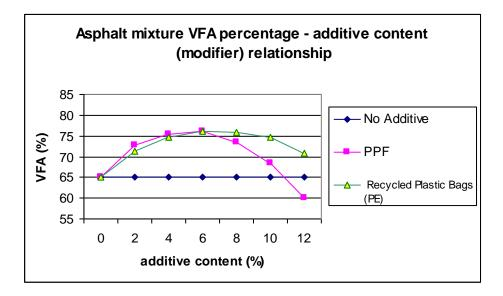
Figure (6) Asphalt Mixture VFA Percentage – Additive Content (Modifier) Relationship.
