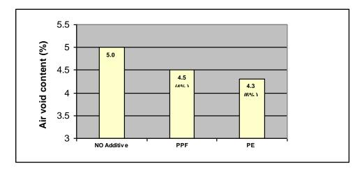
Figure (8) Minimum Asphalt Mixture Air Void Percentage by Type of Modifier.
