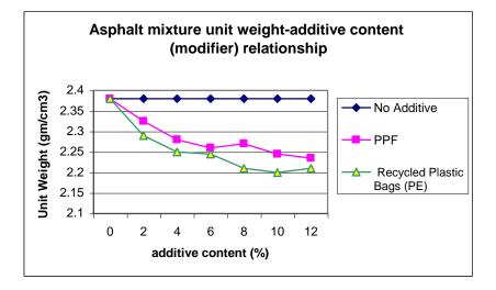
Figure (1) Asphalt Mixture Unit Weight – Additive Content (Modifier) Relationship.
