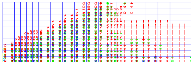
c. Crack pattern for RC beam (CP90II) at load level of 160 kN (P u ).
