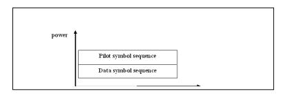
Fig. (1) A frame for superimposed pilot channel estimation
