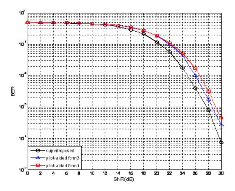
Fig. (6) BER performance of OFDM system based LS estimator for three types of pilot arrangement in 2paths Rayleigh fading channel
