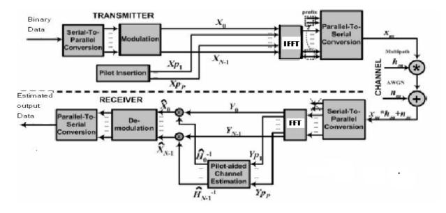
Fig. (4) OFDM system based pilot channel estimation
