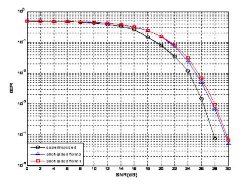
Fig. (5) BER Performance Of OFDM System Based LS Estimator For Three Types Of Pilot Arrangement In Flat Rayleigh Fading Channel
