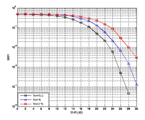
Fig. (13) BER performance of OFDM system based LS estimator with superimposed pilot arrangement and variable time delays in 3-paths Rayleigh fading channel
