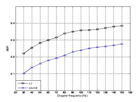
Fig. (12) BER performance of OFDM system based LS and MMSE estimators with superimposed pilot arrangement at SNR=18dB and Doppler frequancies range(30 – 150)Hz in 3-paths Rayleigh fading channel
