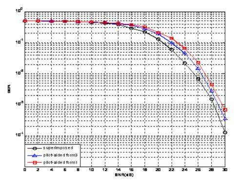
Fig. (7) BER performance of OFDM system based LS estimator for three types of pilot arrangement in 3paths Rayleigh fading channel
