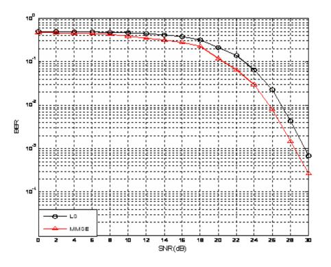
Fig. (10) BER performance of OFDM system based LS &MMSE estimators for pilotaided form(1) arrangement in 3-paths Rayleigh fading channel
