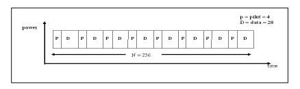
Fig. (2) A frame of conventional pilot assisted channel estimation with N = 256, Q = 8,  $P_i = 32$  and  $N - P_i = 224$ .
