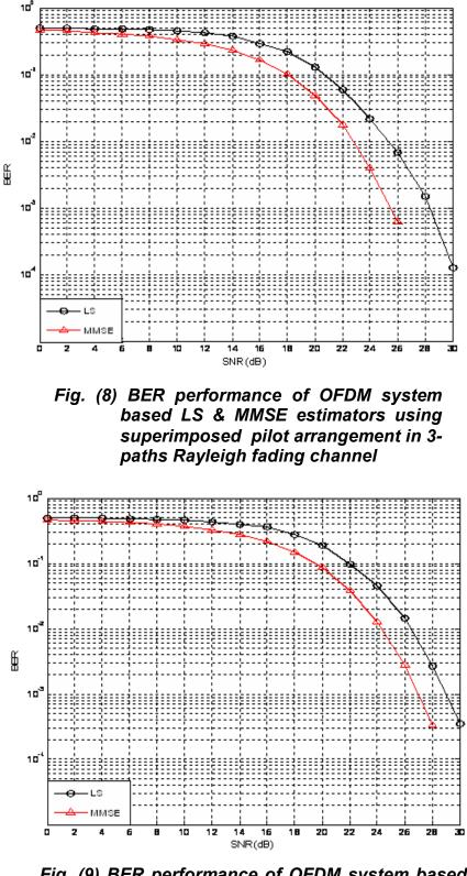
Fig. (9) BER performance of OFDM system based LS &MMSE estimators for pilot-aided form3 arrangement in 3-paths Rayleigh fading channel
