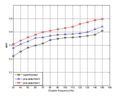
Fig. (11) BER performance of OFDM system based LS estimator for all forms of pilot arrangement at SNR=18dB with Doppler frequancies range (30 – 150) Hz in 3-paths Rayleigh fading channel
