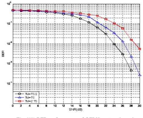
Fig. (18) BER performance of OFDM system based MMSE estimator with pilot -aided form1 arrangement and variable time delays in 3-paths Rayleigh fading channel
