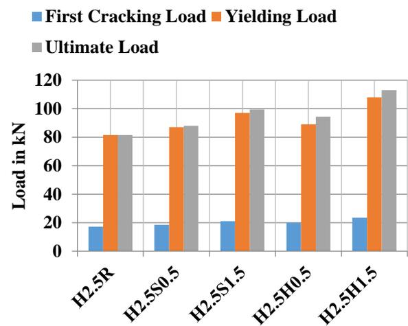
Figure 12. 1st crack load, ultimate strength and yield load levels of group three
