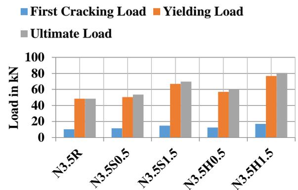
**Figure 9.** 1<sup>st</sup> crack load, ultimate strength and yield load levels of group two
