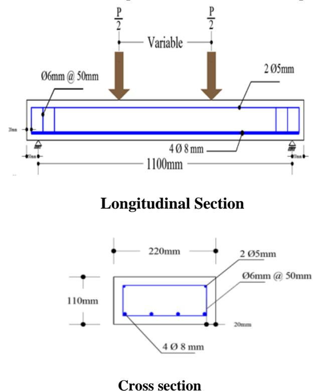
Figure 1. Specimen details of the current study
