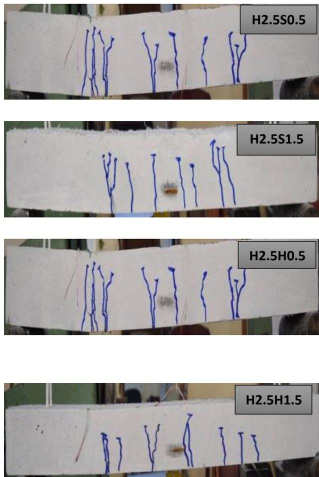
Figure (14) Cracking pattern of group three
