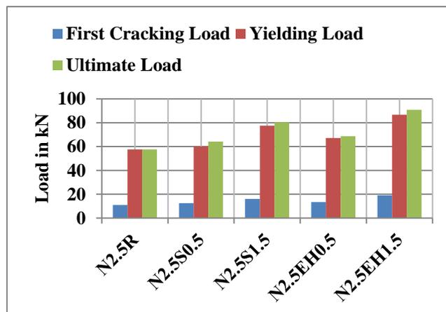
**Figure 6.** Levels of 1st crack load, ultimate strength and yield load of group one
