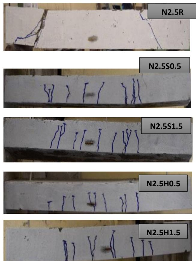
Figure 8. Cracking pattern of group one
