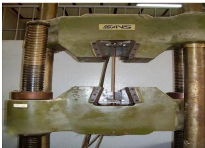
**Figure 2.** Reinforcing bar testing
