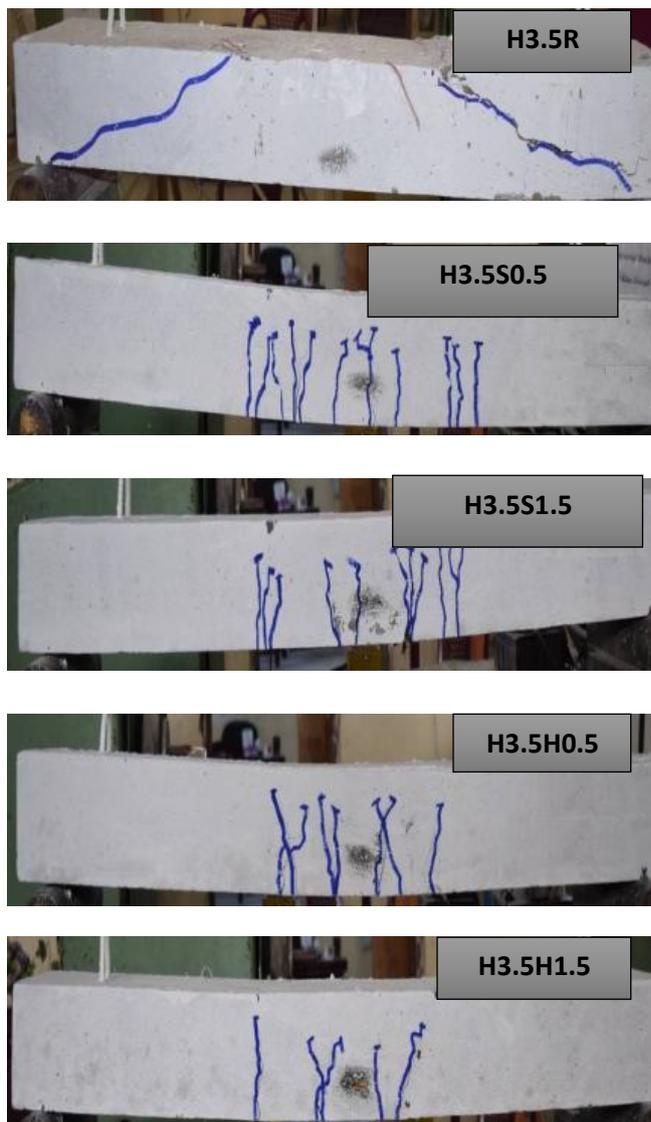
Figure 17. Cracking pattern of group three
