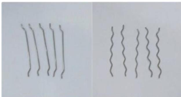
**Figure 4.** The steel fiber used in the present study
