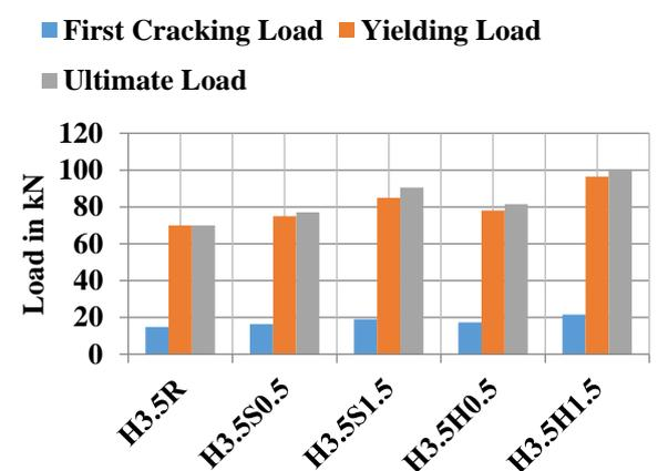
Figure 15. 1st crack load, ultimate strength and yield loading levels of group four
