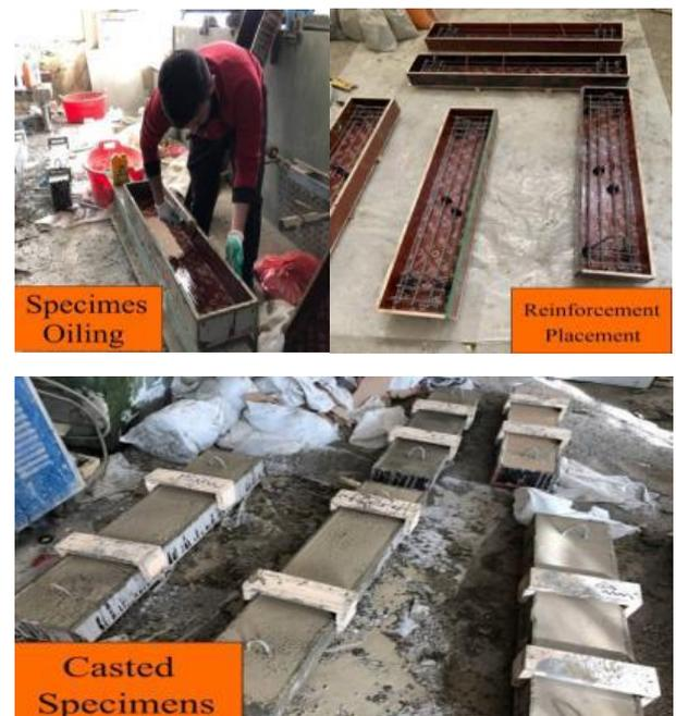
**Figure 3.** Casting procedure
