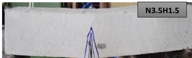
Figure 11. Cracking pattern of group two
