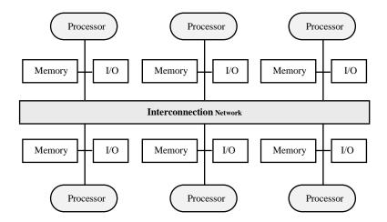
Figure 3: The Non-Uniform Memory Access (NUMA) multiprocessor model.
