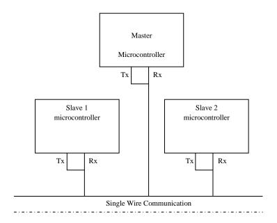
Figure 9: Multi-microcontroller Configuration: Master-Slave connection
