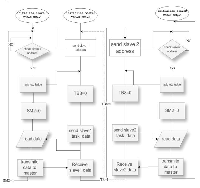
Figure 10: Flow chart for communication protocol for master/slaves communication
