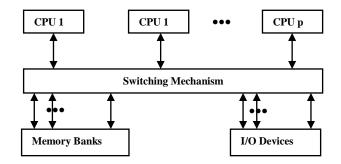
Figure 2: The Uniform Memory Access (UMA) multiprocessor model.
