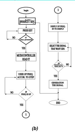
Figure 7 : Signal generator implemented by using one microcontroller
