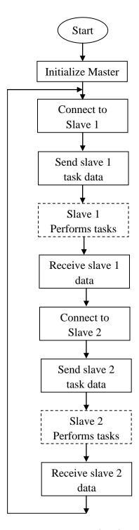
Figure 5: Flowchart for the master communication program of Sequential (non-parallel) processing.
