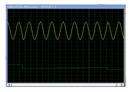
Figure 8 : Signal generator implemented by using parallel processing Sine wave Frequency = 1.14 MHz
