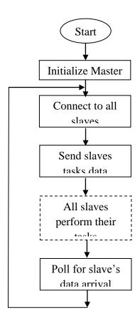
Figure 6: Flowchart for signal generation using parallel processing
