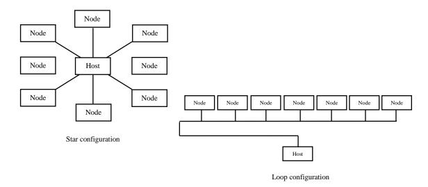
Figure 1: Communications configurations
