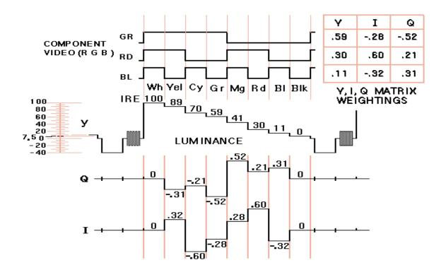
Figure( 8) The Y, I and Q matrix with (RGB) representation in NTSC<sup>[10]</sup>.
