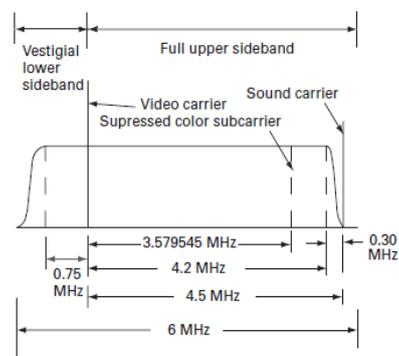
**Figure(7)Vestigial Sideband Modulation<sup>[7]</sup>**
