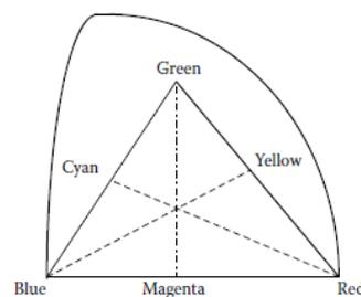
**Figure 2 (b). The spectral locus <sup>[2]</sup>.**
