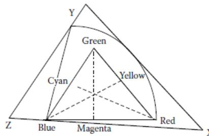
**Figure (3) The CIE theoretical primaries and their relationship to the spectral locus<sup>[2]</sup>.**
