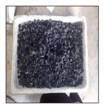
Fig.(1)Waste Tires Particles
