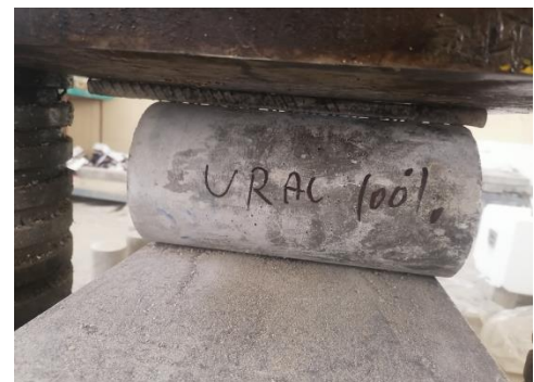
Figure 3. Tensile splitting strength test
