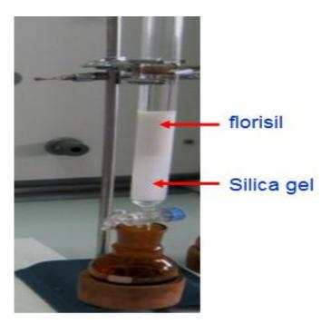
Fig.(5) Purification by chromatographic column
