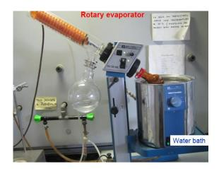
Fig. (3) Rotary evaporator used for evaporation.
