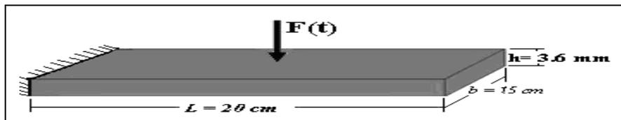
*Figure (6): Cantilever laminate plate*
