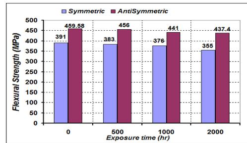
**Figure (5): Variation in the flexure strength of composite symmetric and anti- symmetric laminate due to UV radiation exposure impact.**
