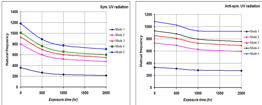
Figure (10) Variation in the natural frequencies with exposure time to UV radiation (a) Symmetric (b) Anti-symmetric (simply supported)
