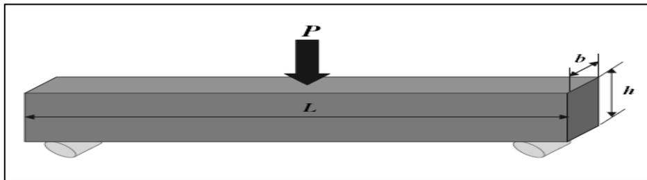
**Figure (1): Schematic drawing of three point bending test**
