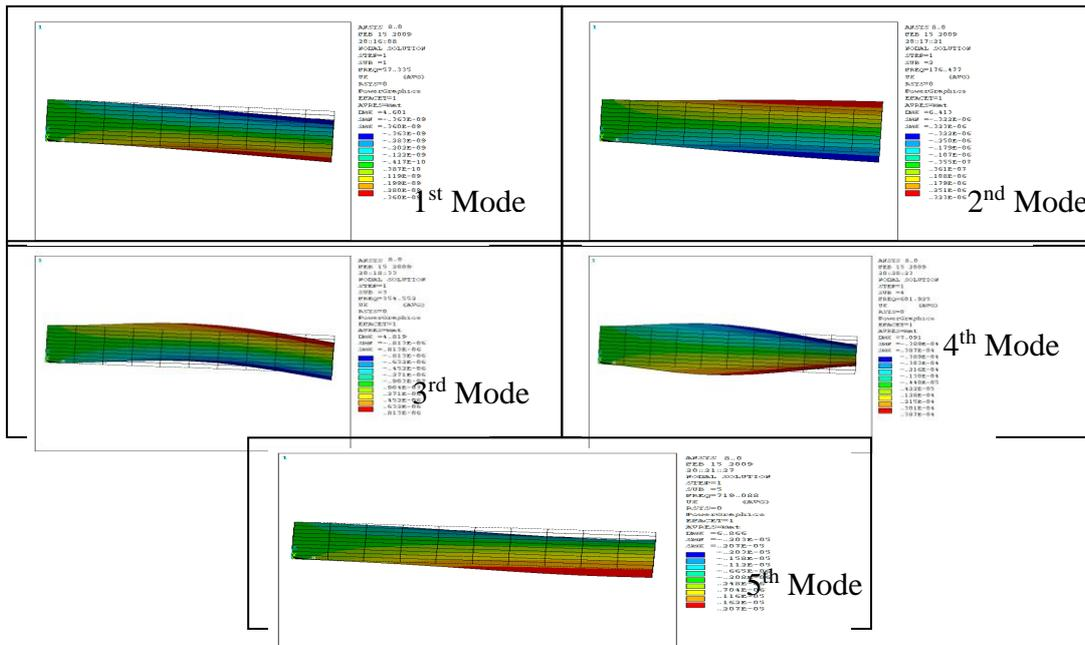
**Figure (8): 1<sup>st</sup>, 2<sup>nd</sup>, 3<sup>rd</sup>, 4<sup>th</sup>, 5<sup>th</sup> mode shapes of symmetric cantilever plate
