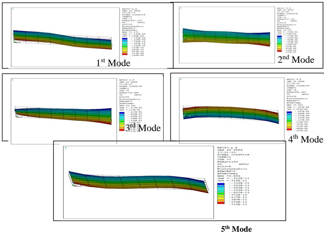
Figure (11) represents the modes of free vibration of symmetric and anti-symmetric simply supported plate for the (1<sup>st</sup>), (2<sup>nd</sup>), (3<sup>rd</sup>), (4<sup>th</sup>) and (5<sup>th</sup>) mode shapes of vibration.
