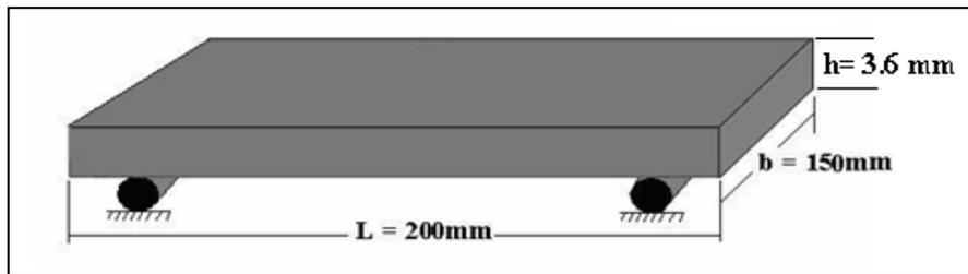
**Figure (9): Simply supported laminate plate.**
