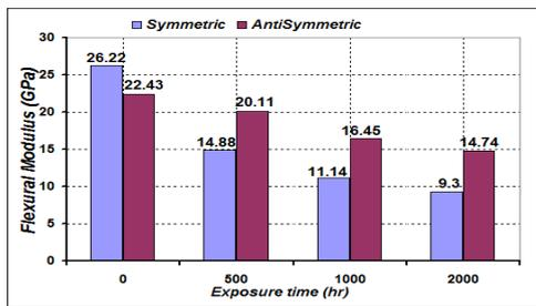
**Figure(4):variation in the flexure modulus Of composite symmetric and ant-Symmetric specimens due to UV radiation Exposure impact.**
