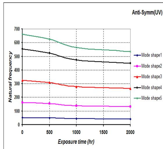
**Figure (7) Variation in the natural frequencies with exposure time to UV radiations (a) symmetric (b) anti-symmetric (cantilever plate) .**
