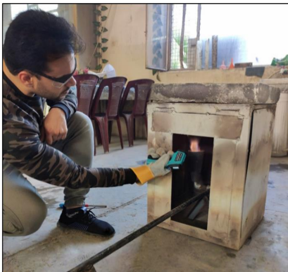
Figure 7. Taking average temperature for concrete
