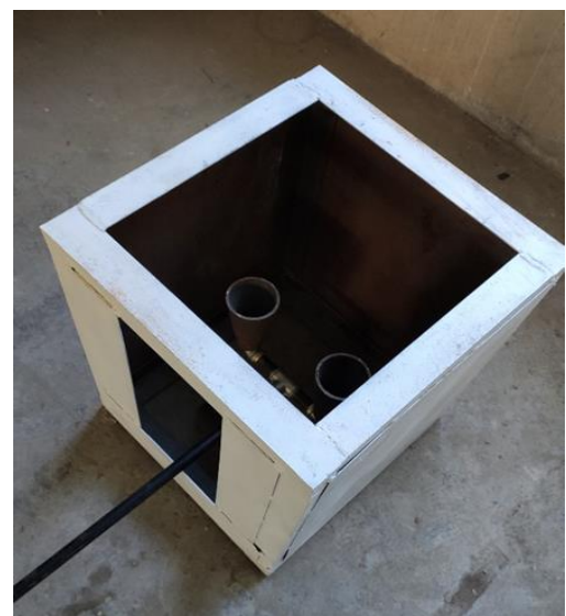
Figure 5. Steel frame with burner
