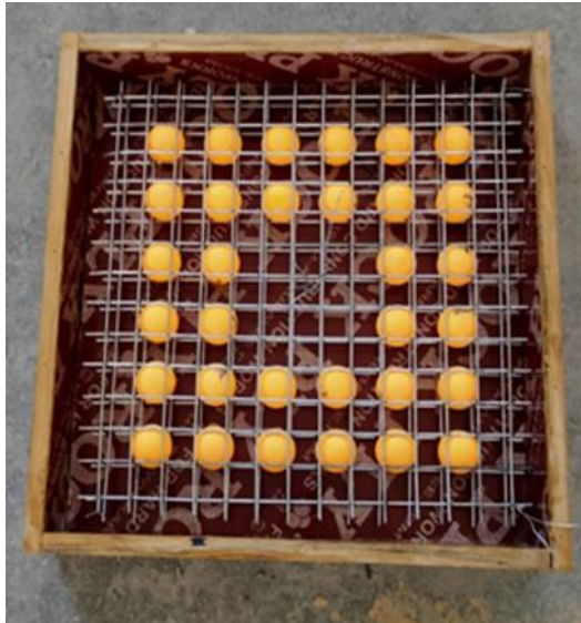
Figure 2. Plywood mold with steel reinforcement
