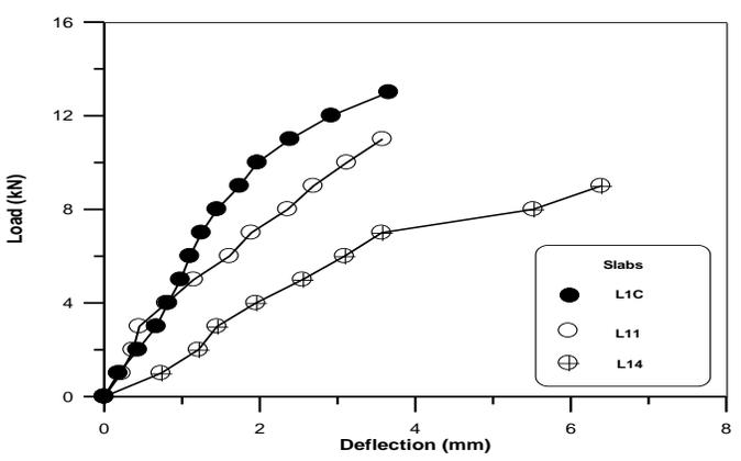
Figure (12) Load –Deflection relationship for LWC punching slab specimens at different temperature levels.
