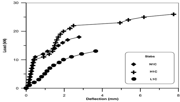
Figure (6) Load –Deflection relationship for punching slab specimens N1C, H1C and L1C (room temperature conditions).
