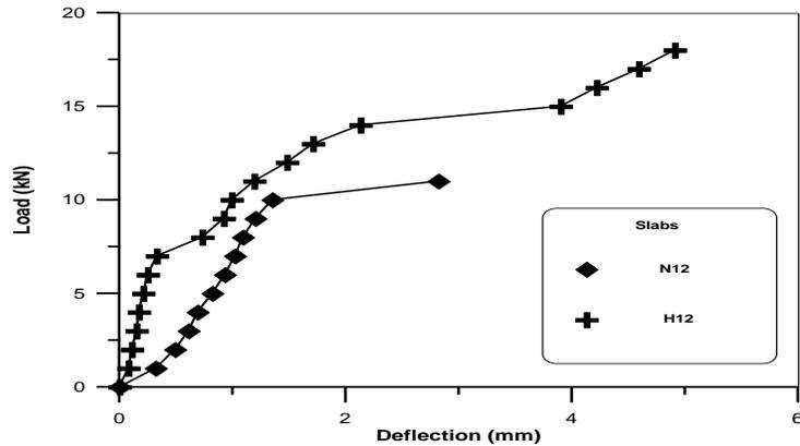
Figure (8) Load –deflection relationships for punching slab specimens N12 and H12 (450° C).
