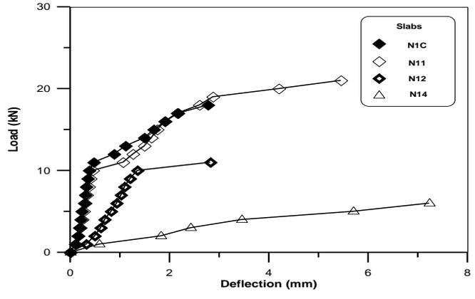
Figure (10) Load –Deflection relationship for NSC punching slab specimens at different temperature levels.
