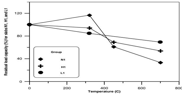
Figure (5) Effect of high temperature on the residual load capacity for the punching groups of slab specimens
