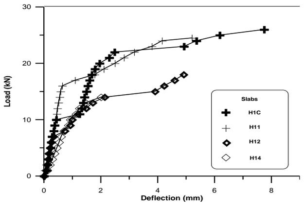
Figure (11) Load–Deflection relationship for HSC punching slab specimens at different temperature levels.
