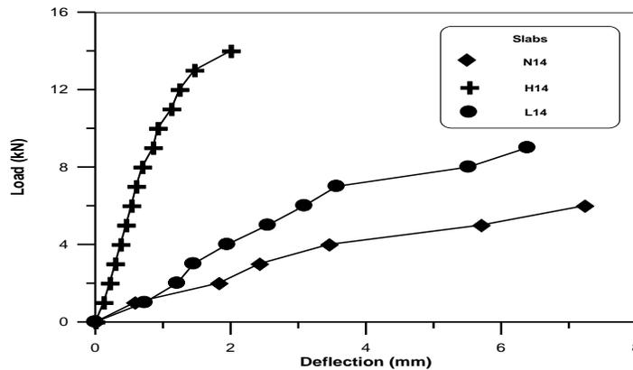
**Figure (9) Load –deflection relationships for punching slab specimens N14, H14 and L14 (700 ° C).**
