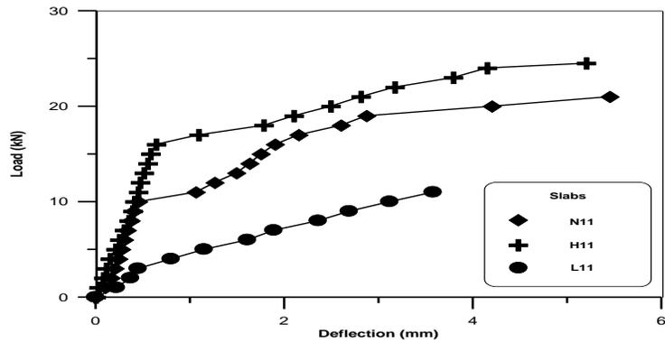
Figure (7) Load-Deflection relationships for punching slab specimens N11, H11 and L11 (320C.)
