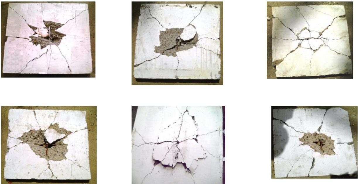
**Figure (13) Some of slab specimens of groups N1, H1 and L1**
