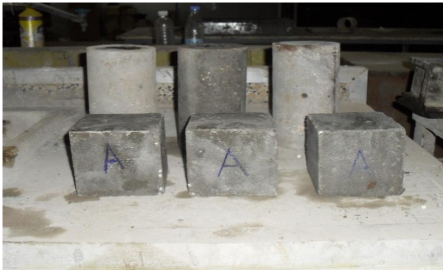
Fig (3)sample of cubes and cylinders of SC-PC (mix A)
