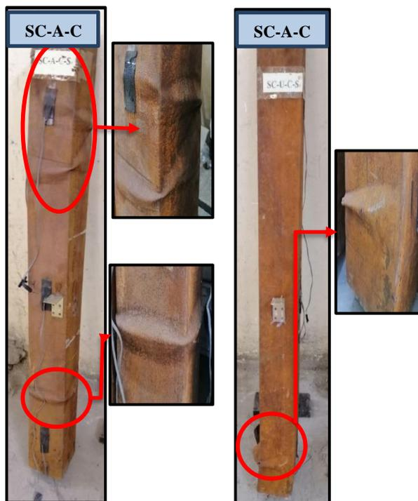
Figure 20. Buckling Pattern for (SC-A-C) and (SC-U-C)
