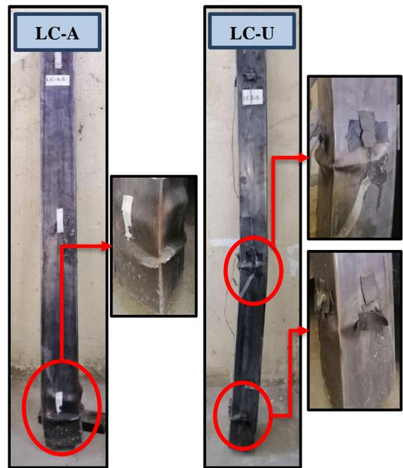
**Figure 17.** Buckling Pattern for (LC-A) And (LC-U)
