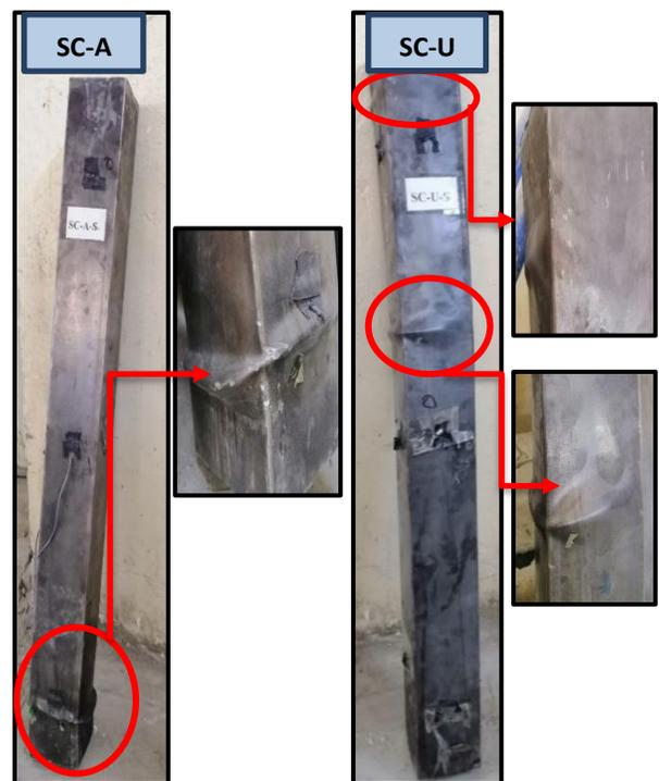
**Figure 18.** Buckling Pattern for (SC-A) and (SC-U)
