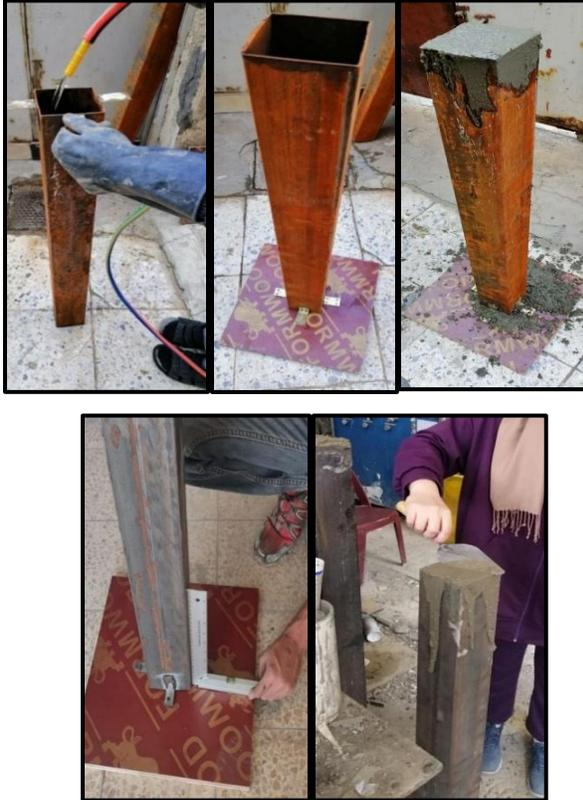
**Figure 5.** The concrete casting for the specimens tested
