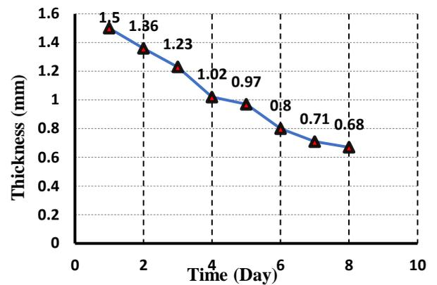
Figure 4. corrosion rate and a decrease in steel section thickness
