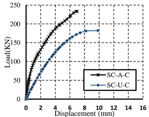
**Figure 16.** Load-deflection curves for specimens (SC-A-C) and (SC-U-C)
