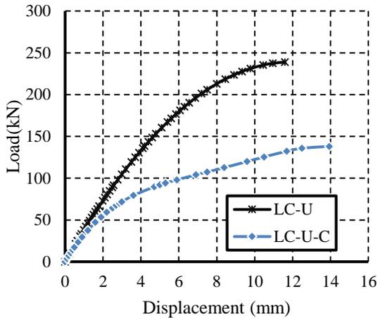
**Figure 12.** Load-deflection curves for uniaxially loaded specimens (LC-U) and (LC-U-C)
