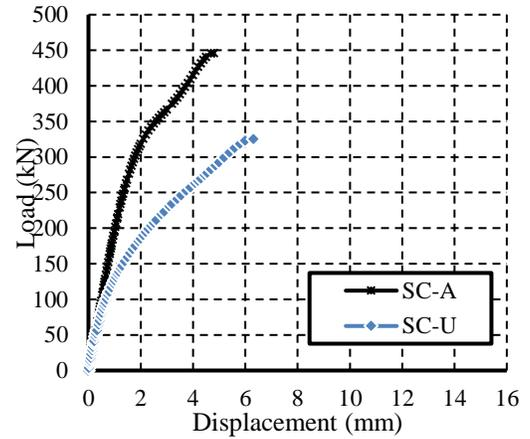
**Figure 15.** Load-deflection curves for specimens (SC-A) and (SC-U)
