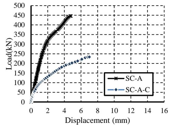
**Figure 9.** Load-deflection curves for axially loaded specimens (SC-A) and (SC-A-C)
