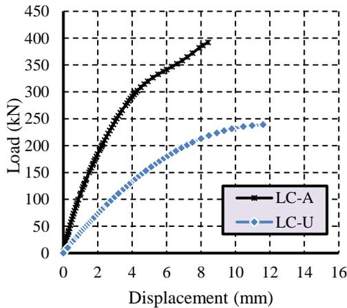
**Figure 13.** Load-deflection curves for specimens (LC-A) and (LC-U)
