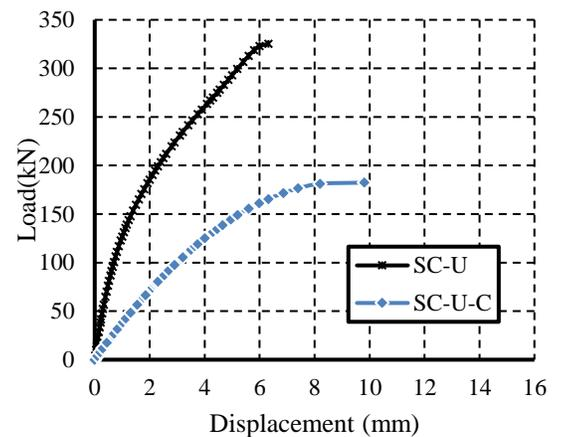
**Figure 10.** Load-deflection curves for uniaxially loaded specimens (SC-U) and (SC-U-C)
