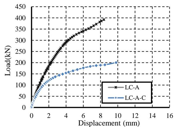
**Figure 11.** Load-deflection curves for axially loaded specimens (LC-A) and (LC-A-C)
