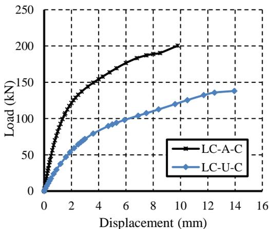
**Figure 14.** Load-deflection curves for specimens (LC-A-C) and (LC-U-C)
