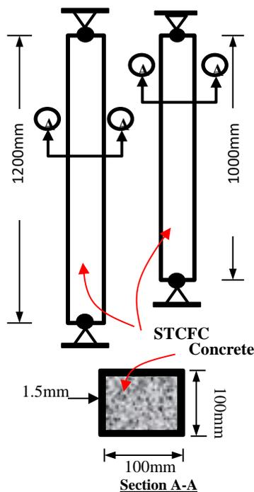
**Figure 1.** Details of the Tested STCFC
