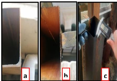
Figure 3. Steel tubular columns: (a) before corrosion; (b) after corrosion; (c) Thickness measured by digital vernier
