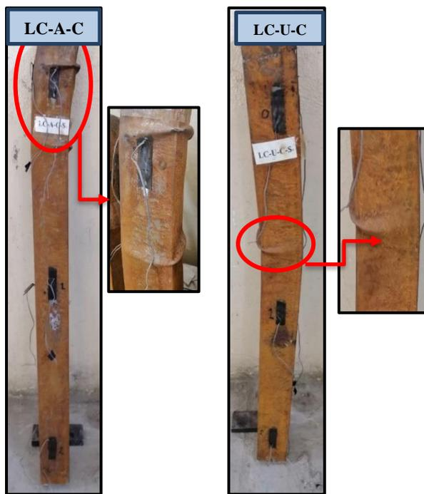
Figure 19. Buckling Pattern for (LC-A-C) And (LC-U-C)
