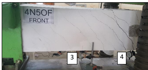
Figure 9. Locations of dial gauges, Twist angle (1,2 left end - 5,6 right end - 3 quarter span - 4 mid span), longitudinal elongation (7, 8).
