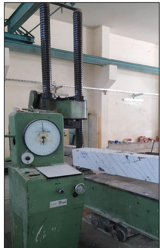
Figure 8. Hydraulic universal testing machine.
