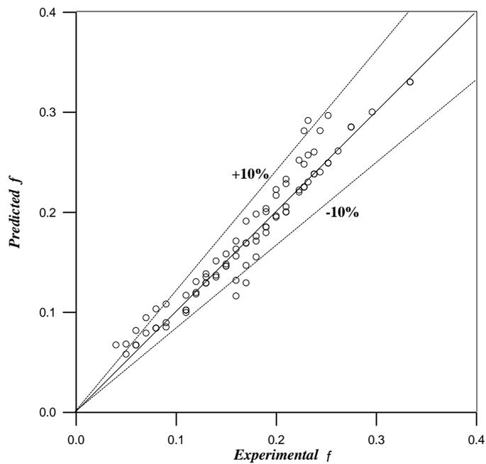
(Figure: 11) Comparison between experimental and predicted friction factor
