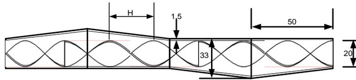
(b) Dimensions of Eccentric Converging-Diverging with twisted tape (in mm)
