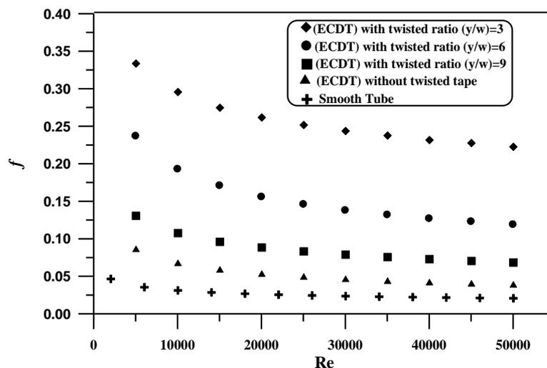
(Figure: 9) Effect of twist ratio on friction factor for (a)  $y/w=3$ , (b)  $y/w=6$ , and  $y/w=9$
