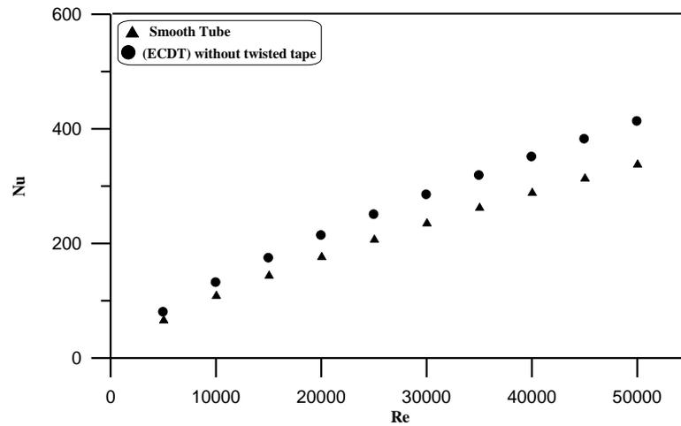
(Figure: 6) Comparison of experimental data of the plain tube and (ECDT) without twisted tape insert for Nusselt number
