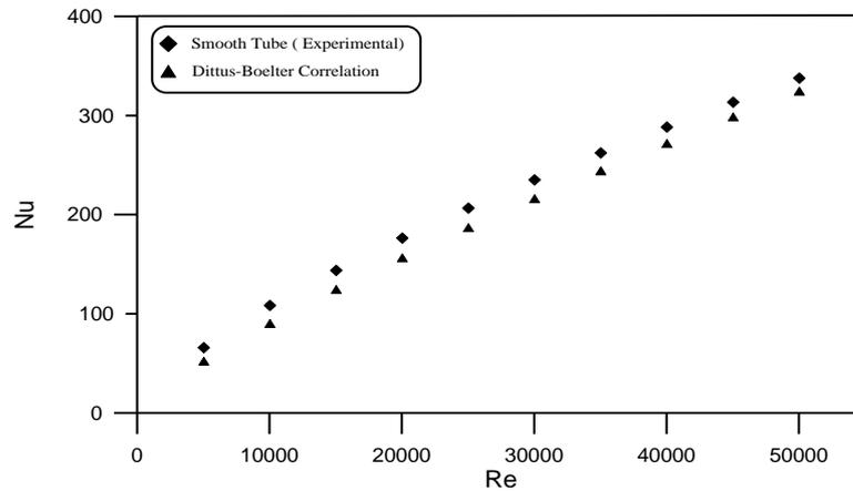
(Figure: 4) Comparison of experimental data and empirical correlation of the plain tube for Nusselt number
