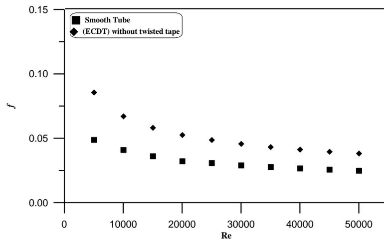
(Figure: 7) Comparison of experimental data of the plain tube and (ECDT) without twisted tape insert for friction factor
