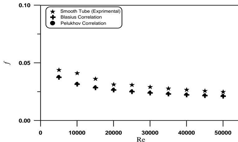
Figure: 5) Comparison of experimental data and empirical correlation of the plain tube for friction factor
