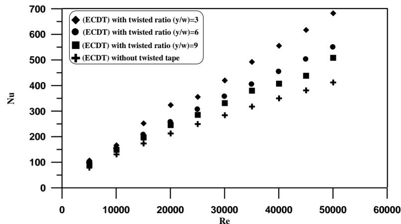
(Figure: 8) Effect of twist ratio on Nusselt Number for (a)  $y/w=3$ , (b)  $y/w=6$ , and  $y/w=9$
