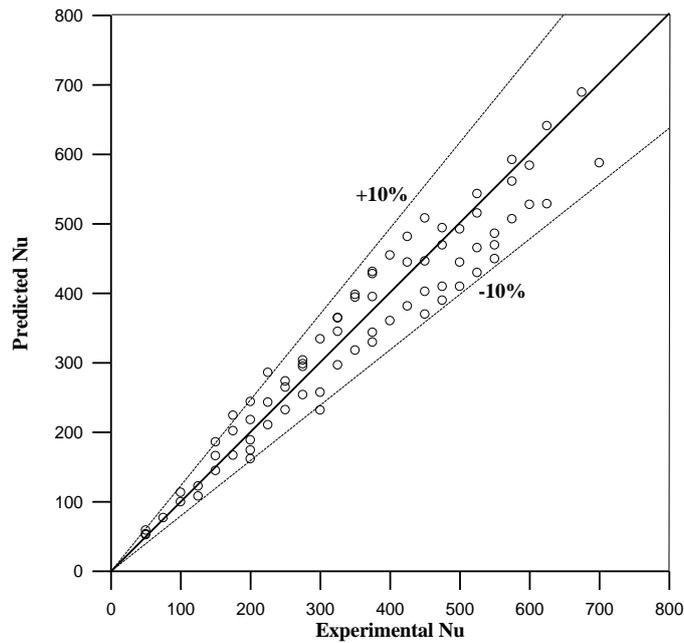
(Figure: 10) Comparison between experimental and predicted Nusselt Number
