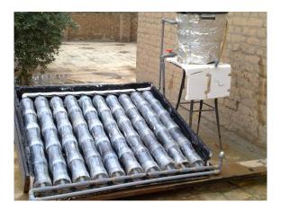
Fig.7: The solar collector
