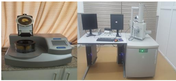
Plate3. Scanning Electronic Microscopy (SEM) with Sputter Coating Device (Microscopic Laboratory, College of Science, University of Kufa)
