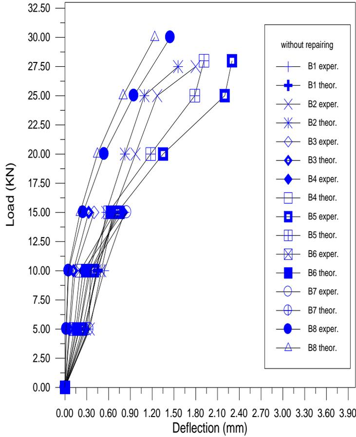
**Fig (8) load – deflection curve for beams without repairing plate**
