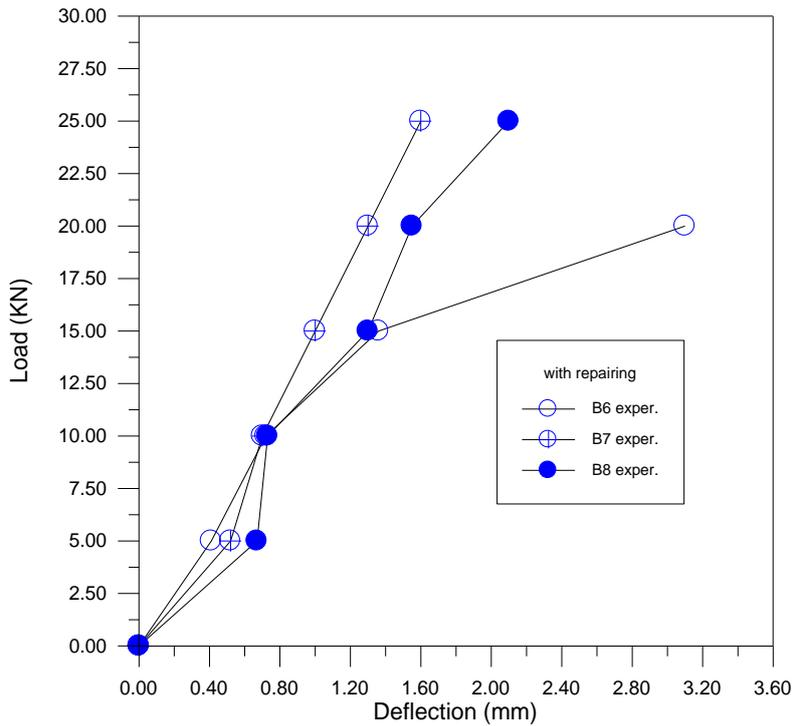
**Fig. (10) load deflection curve for beams with plate reinforcement (with repairing).(tested results)**
