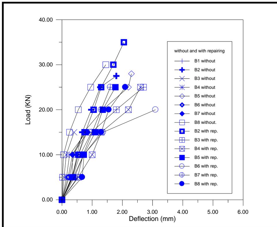
**Fig (12) load – deflection curve for beams with and without repairing plate**
