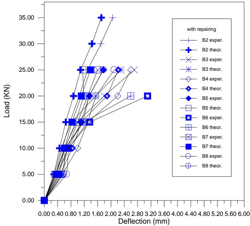
**Fig (11) load – deflection curve for beams with repairing plate**
