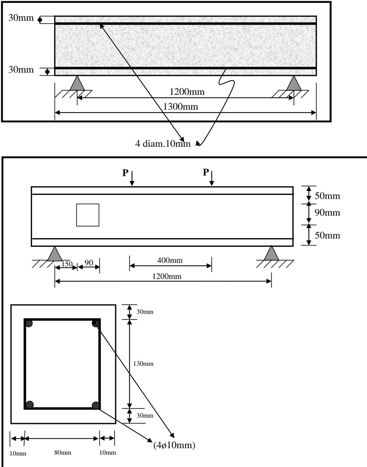
**Fig. (2) the tested reinforced concrete beam with and without opening**
