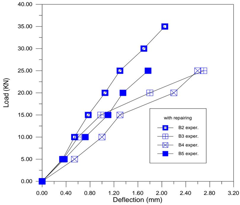
**fig (9) load deflection curve for beams with stirrups (with repairing) (tested results)**
