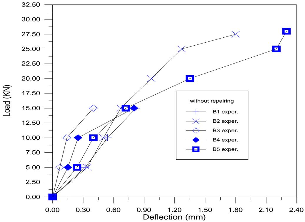
**Fig (6): load deflection curve for beams with stirrups (tested results)**
