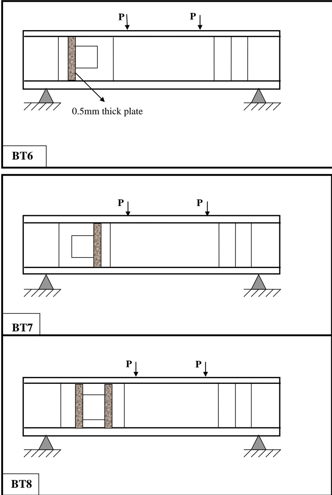
*Fig (4) Reinforced concrete beams using a repairing steel plate*
