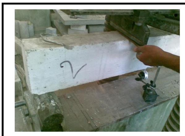
*Two point load applied to beams*
