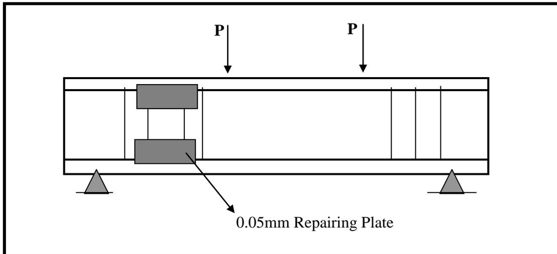
*Fig. (5) Repairing plate for all tested beams .*
