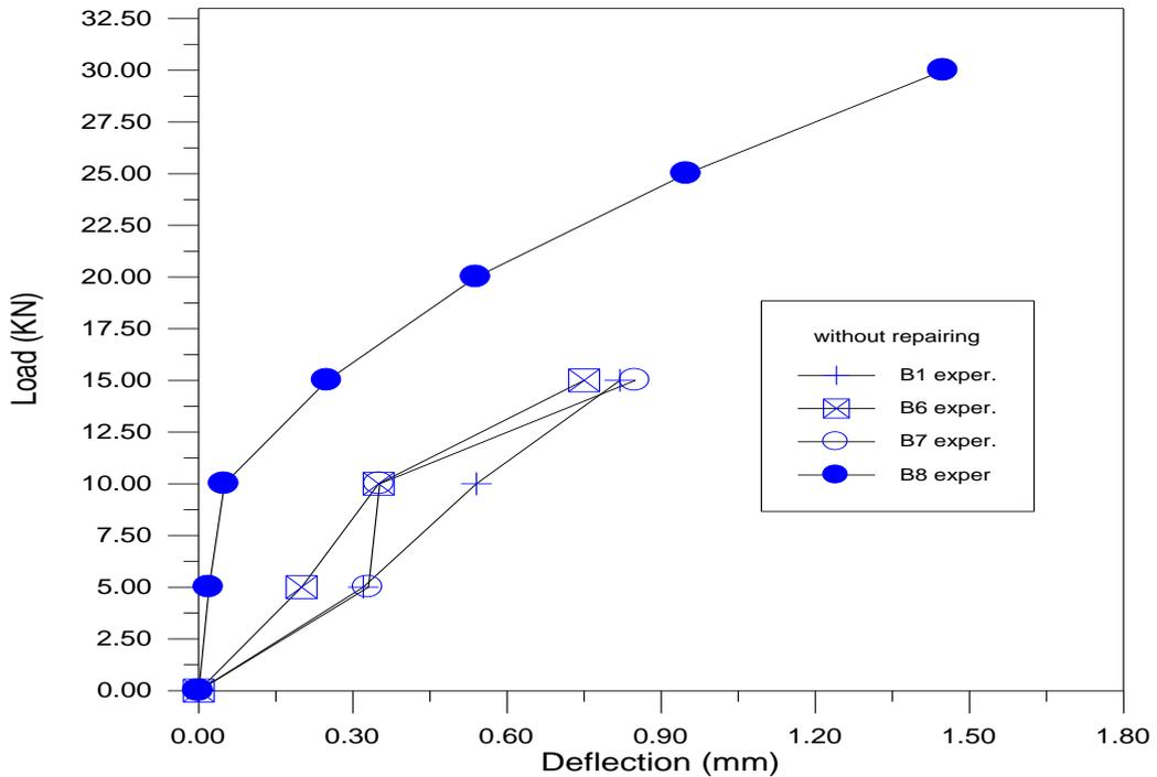
**Fig (7) load deflection curve for beams with plate reinforcement. (tested results)**
