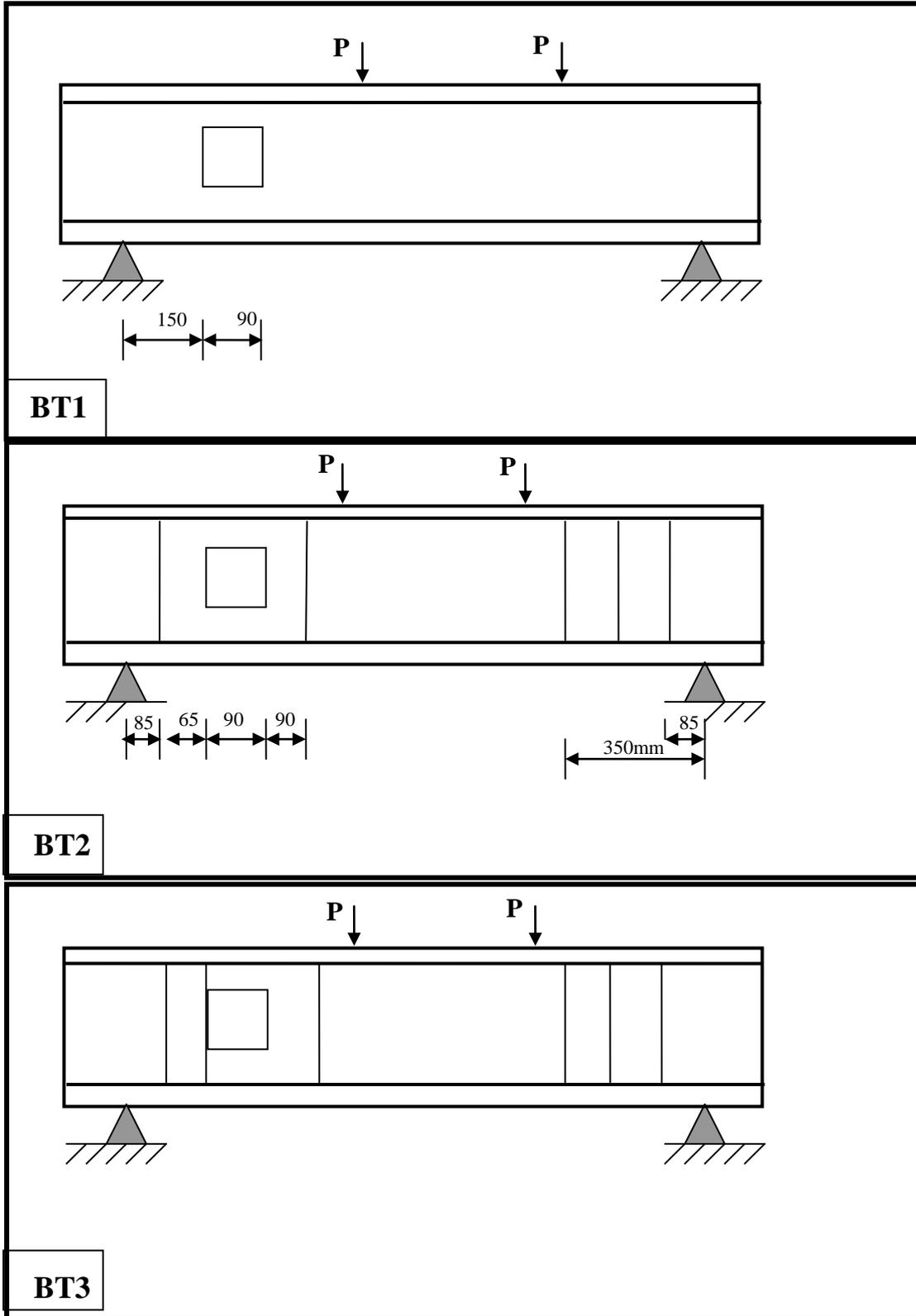
Fig. (3a) Reinforced concrete beams without repairing plate
