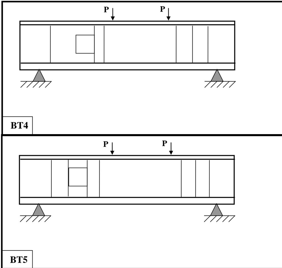
*Fig.(3b) Reinforced concrete beams without repairing plate*
