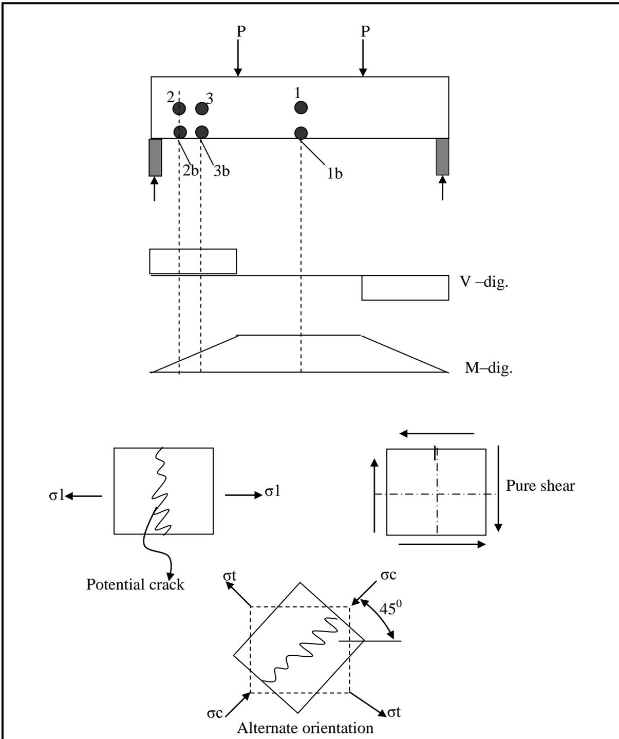
**Fig (1) Cracking Behavior of Concrete due to Shear Loading**
