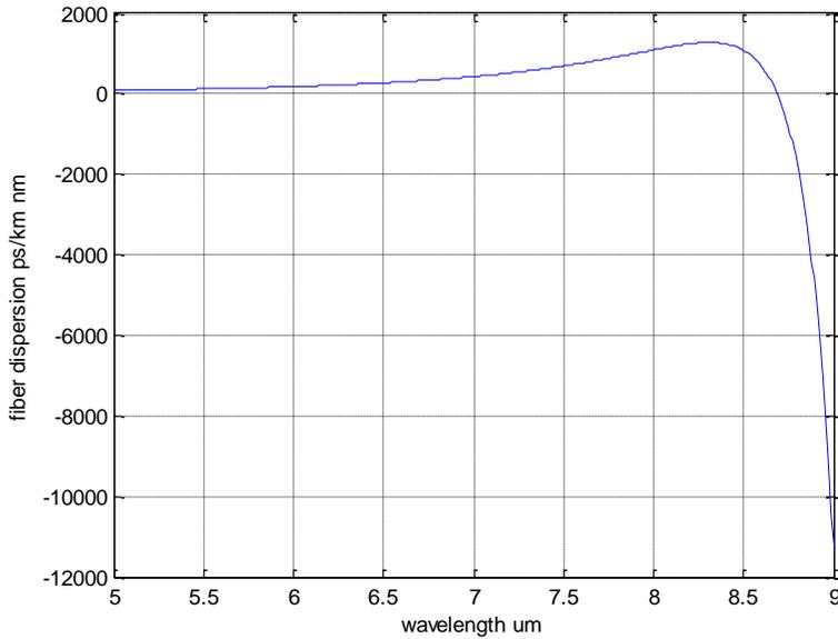
**Figure (5) The maximum  $D(\lambda)$  at the range  $(5-9)\mu\text{m}$  of  $\text{SiO}_2$  fiber**
