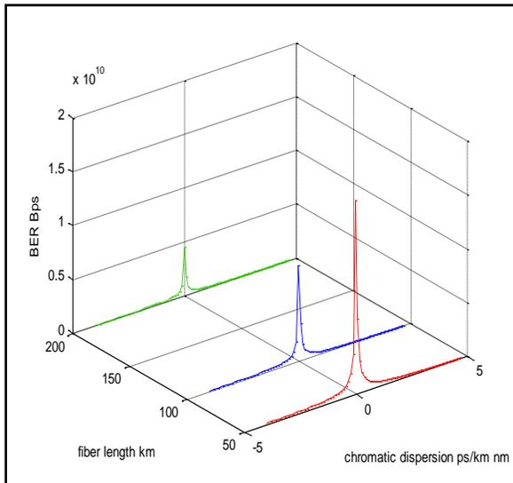
**Figure (3) The relation in 3-D between chromatic dispersion and Bit error rate and fiber length of SiO<sub>2</sub> fiber**
