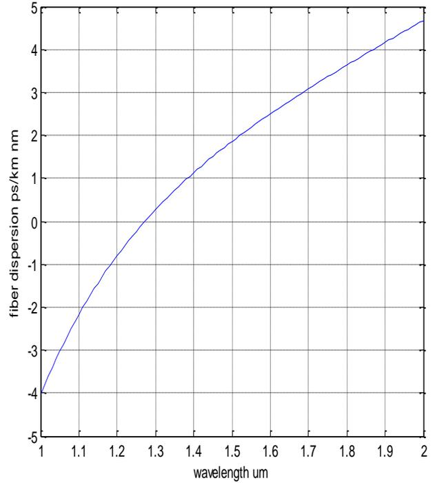
**Figure (2) The relation between the wavelength and chromatic dispersion of SiO<sub>2</sub> fiber**
