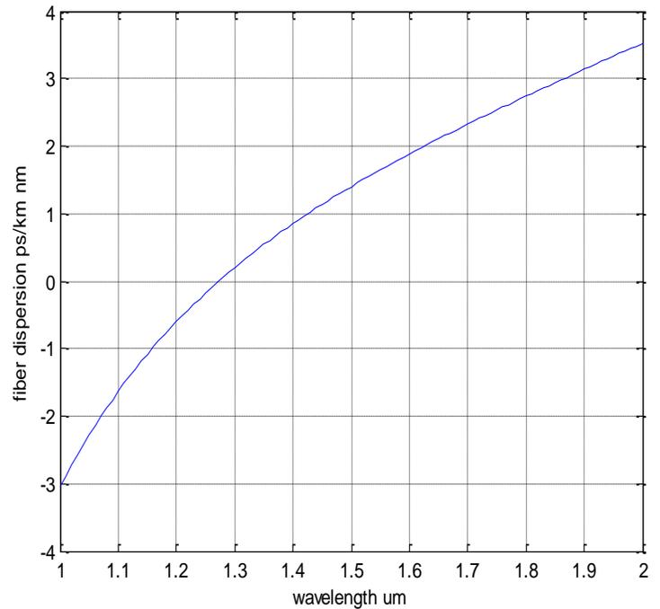
**Figure (8) The relation between the wavelength and chromatic dispersion of  $\text{GeO}_2$  fiber**
