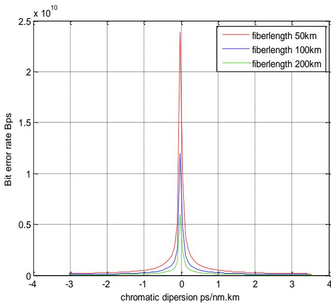
**Figure (7) The relation between dispersion and Bit error rate of  $\text{GeO}_2$  fiber**
