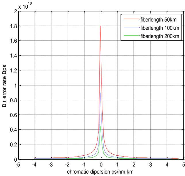
**Figure (1) The relation between dispersion and Bit error rate of SiO<sub>2</sub> fiber**
