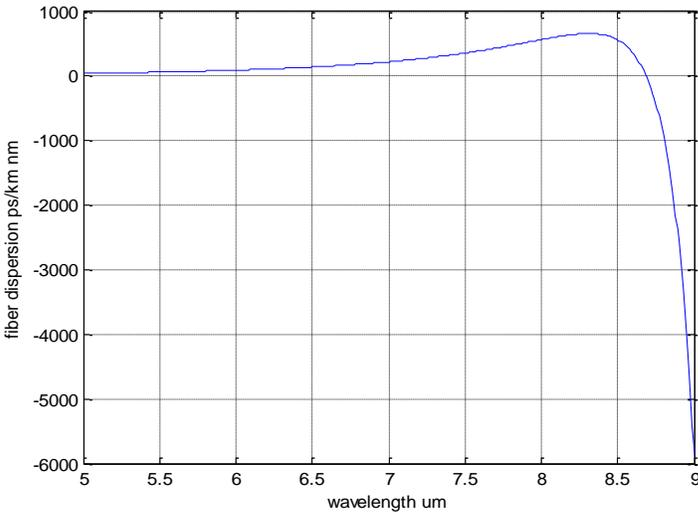
**Figure (11) The maximum  $D(\lambda)$  at the range (5-9)μm of GeO<sub>2</sub> fiber**
