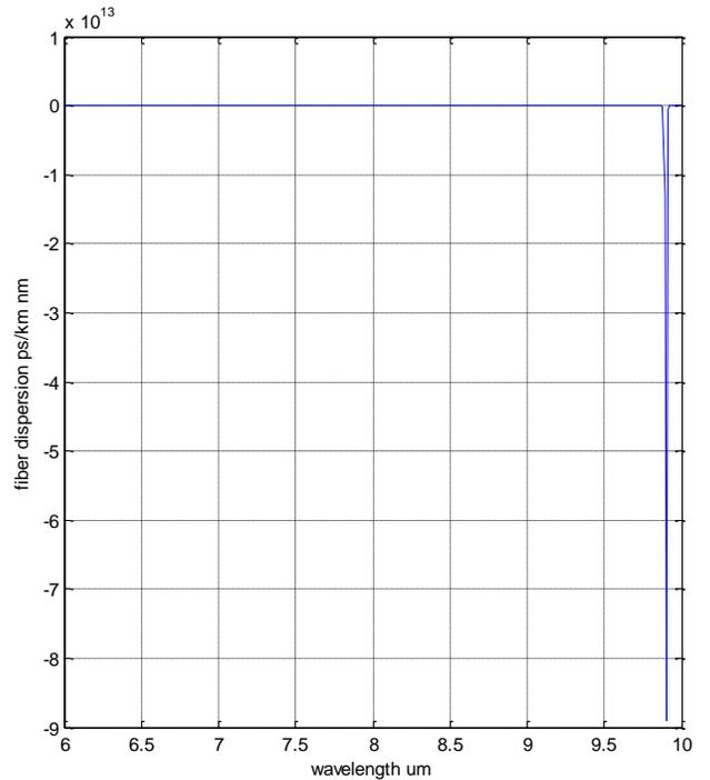
**Figure (12) The minimum  $D(\lambda)$  at the range (6-10)μm of GeO<sub>2</sub> fiber**
