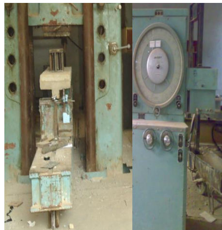
Plate 3: The universal testing machine (8551M.F.L.system ) with a typical beam.
