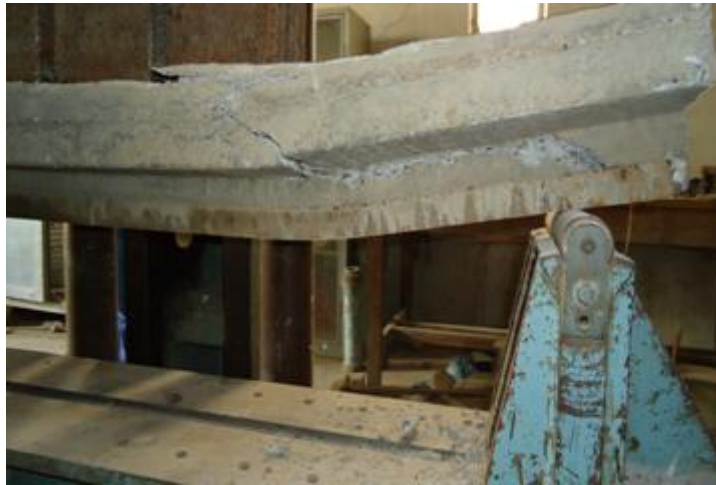
Plate 4: View of a typical tested beam after failure showing the fracture pattern.
