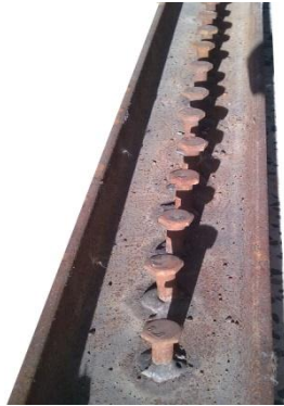
Plate 1: Typical steel channel with its welded headed studs for a typical tested beam
