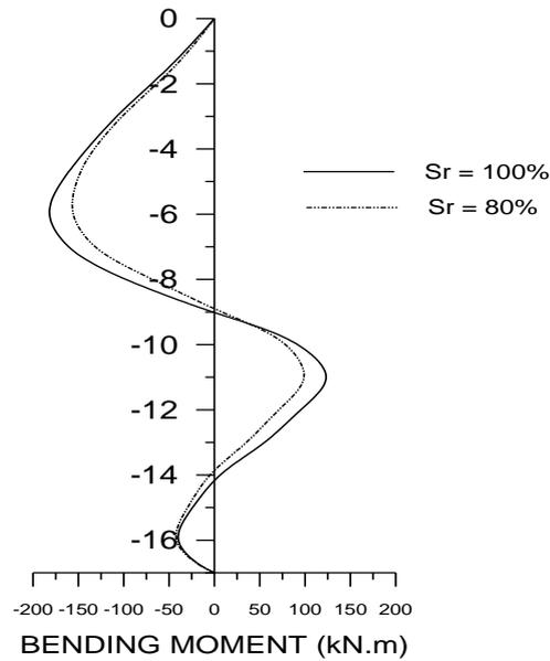
**Figure (5): Predicted wall bending moment for different degrees of saturation.**
