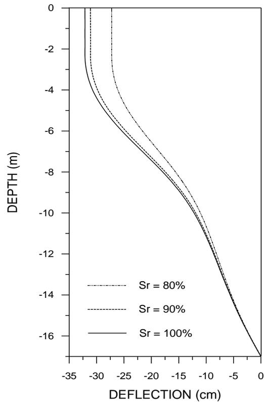
**Figure (4): Lateral movement predicted of the wall for different degrees of saturation.**
