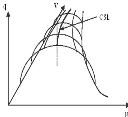
**Figure (1): State boundary surface for modified Cam clay model.
