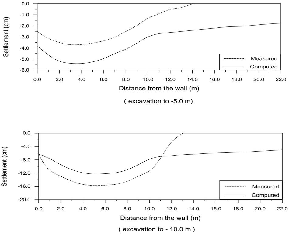
**Figure (17): Comparisons of predicted surface movement with observed values.**
