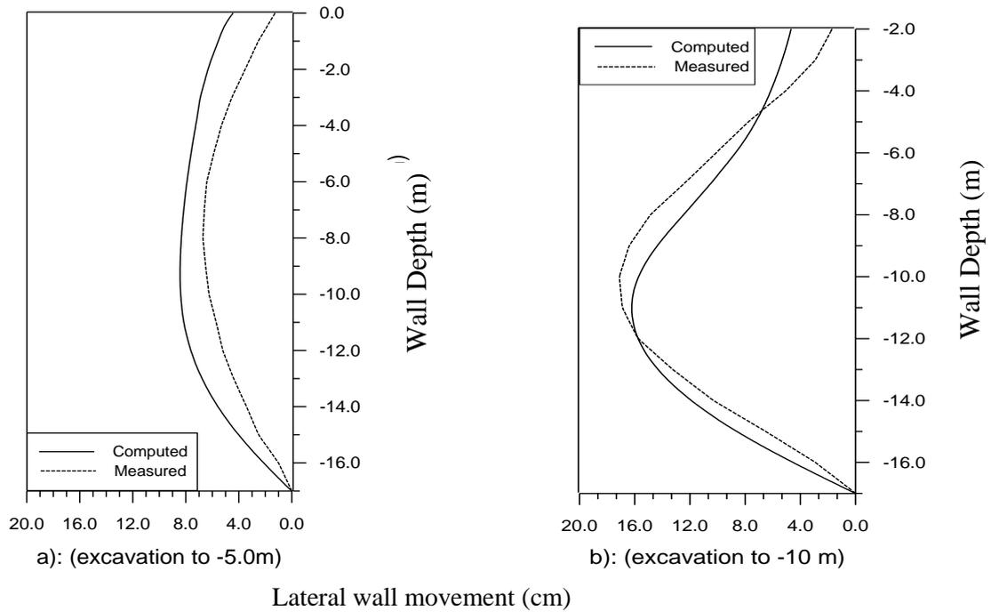
**Figure (16): Comparisons of predicted wall deflection with observed values.**
