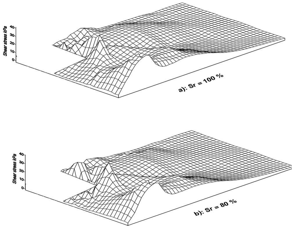
**Figure (12): Predicted shear stresses in the soil in the case of supported excavation with strut at the end of excavation.**
