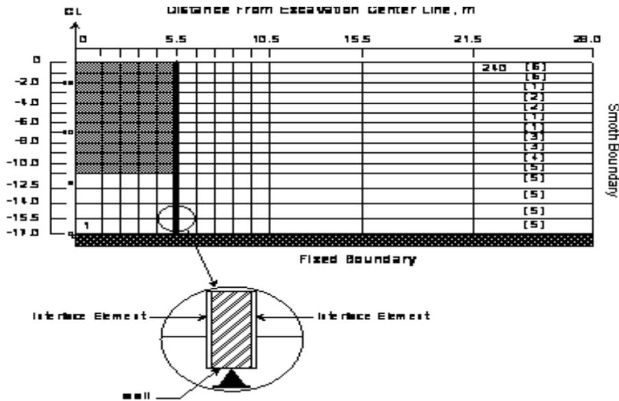
Figure (14): Finite element mesh for real supported excavation in soft clay.
