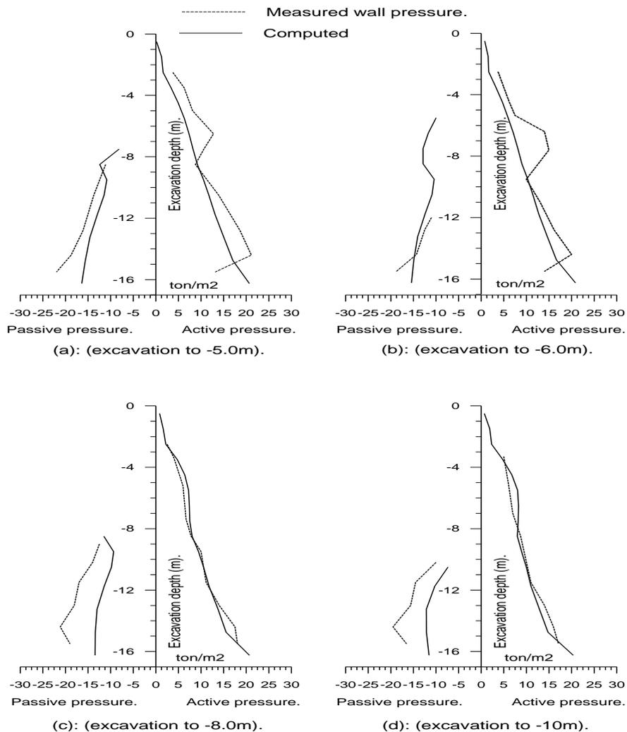
**Figure (15): Comparisons of predicted nonlinear analysis and observed wall pressures.**
