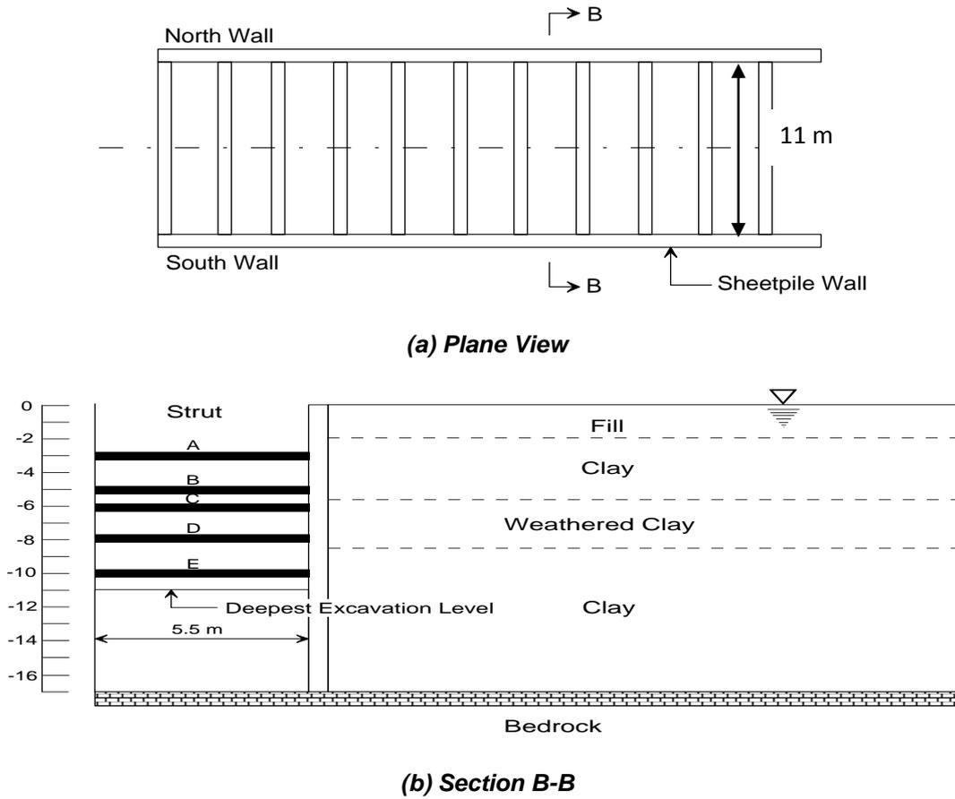
Figure (13): Plane view and detail of real supported excavation in soft clay.
