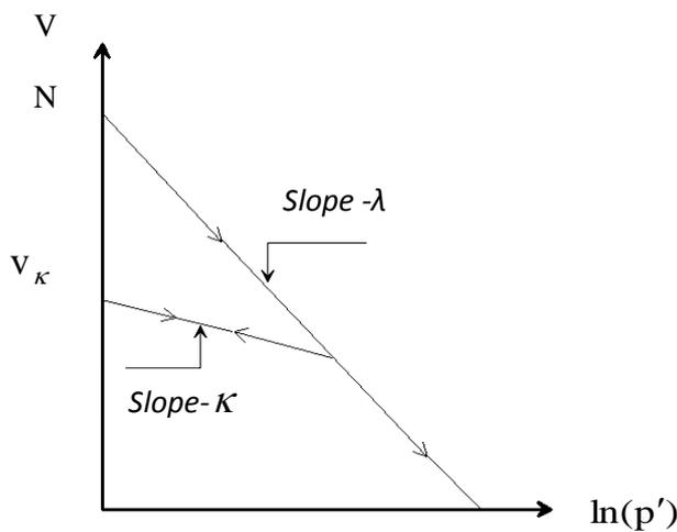
**Figure (2): Identical  $(\ln p', v)$  plot in critical state theory (after Britto and Gunn (1987))**
