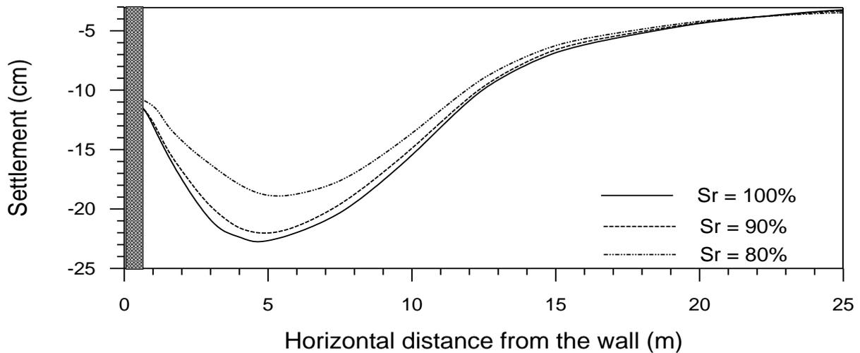
**Figure (6): Surface movement predicted of the soil for different degrees of saturation.**
