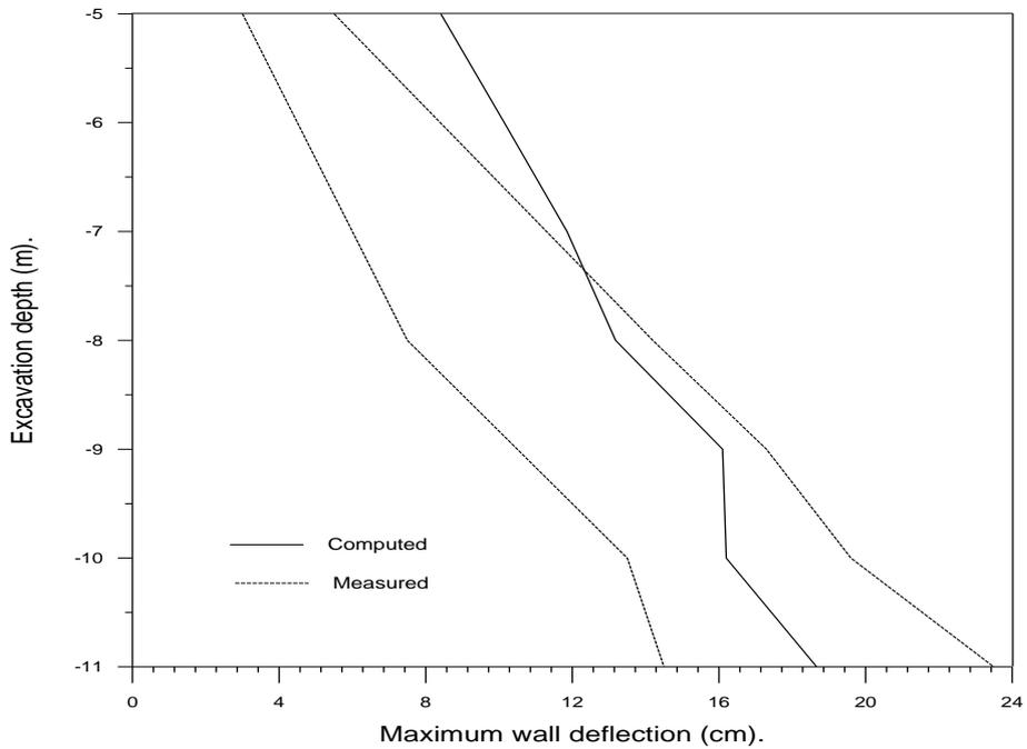
**Figure (18): Comparisons of predicted maximum wall deflection with range of measured values.**
