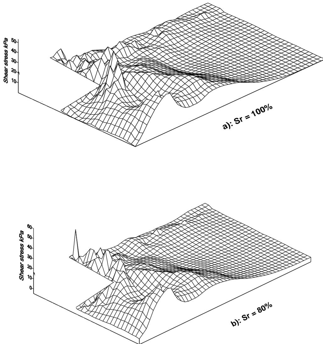
**Figure (8): Predicted shear stresses in the soil at the end of excavation.**
