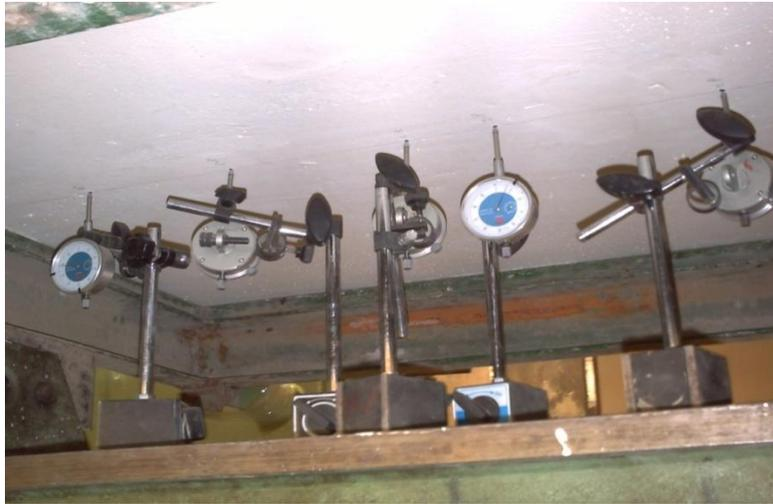
Plate (4) Deflection Measurement at Tension Face of Specimens
