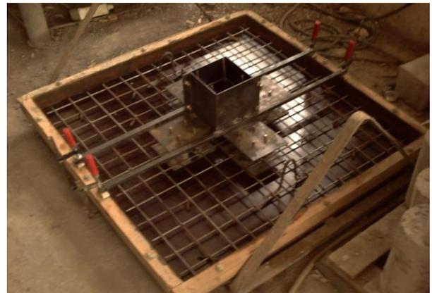
**Plate (2) Slab Mould**
