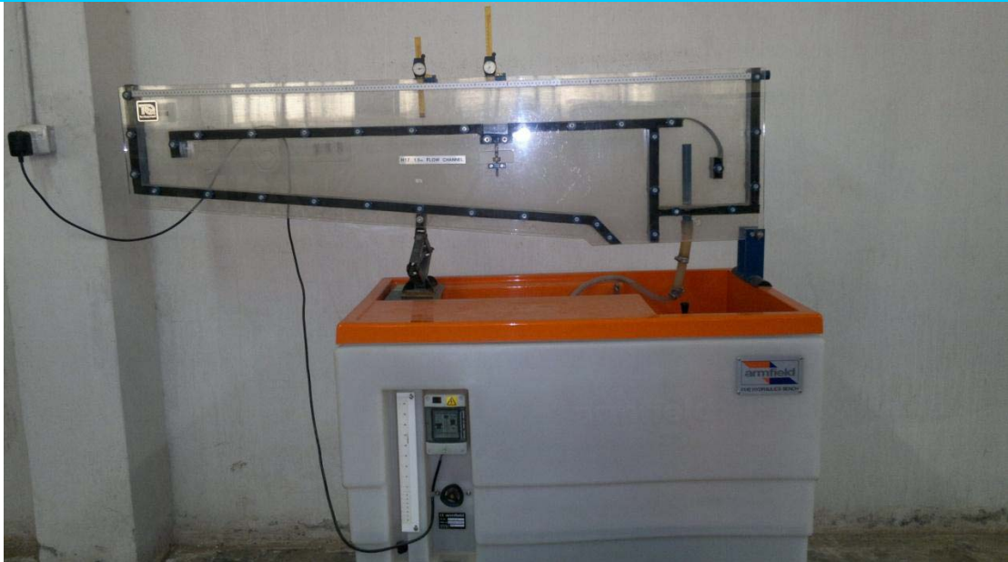
Fig.(1 ): 1.5m ,52mm-open channel flume &Armfield, F1-10Hydr. Bench.
